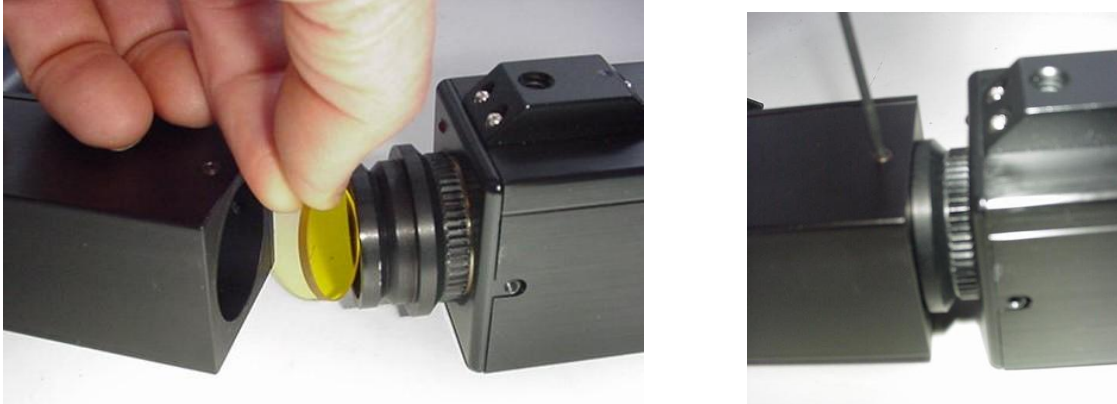
Figure 6: a) blocking filter placed in C-mount; b) attaching C-mount to spotting scope.
