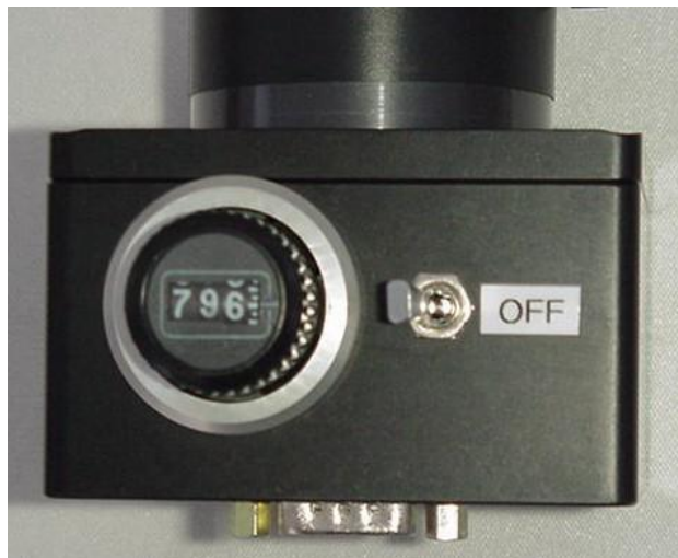
Figure 7: Quadrant PMT controls.
