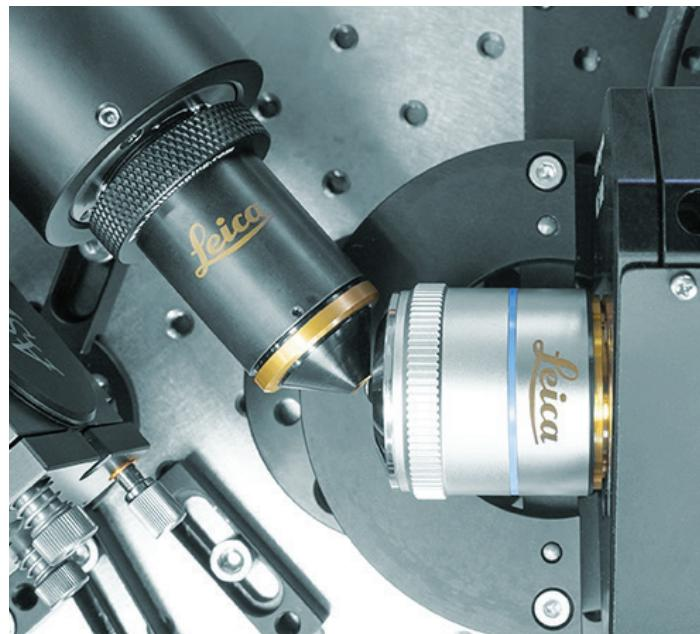
The single-objective light sheet geometry – known in the literature as OPM, SCAPE, SOPi, eSPIM, and SOLS – enables 4D fluorescence imaging of biological samples at high speed and low light dose with conventional sample mounting. Previously such a microscope had to be home-built; now ASI is making this transformative technology broadly available in collaboration with Leica Microsystems.
