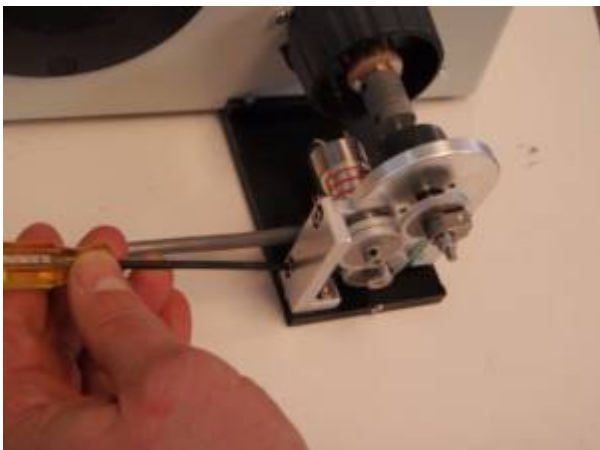
Tighten the vertical adjustment screws after alignment.
