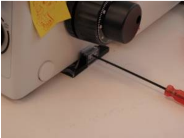
Tighten the baseplate clamp snugly.
