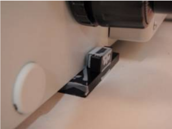
Leave base plate clamp loose at this time.
