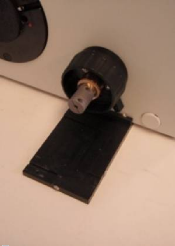
Slide base plate under microscope and center beneath focus assembly.
