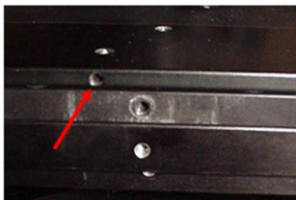
Insert's setscrew access on right side of stage.
