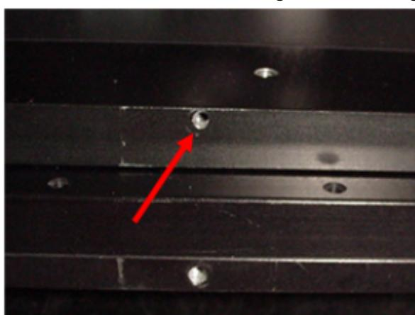
Insert's setscrew access on rear of stage.
