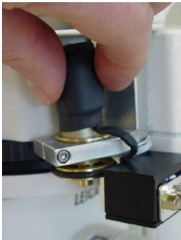
Figure 7: Loosen clamp and rotate motor clockwise to engage the rubber wheel with the filter turret
