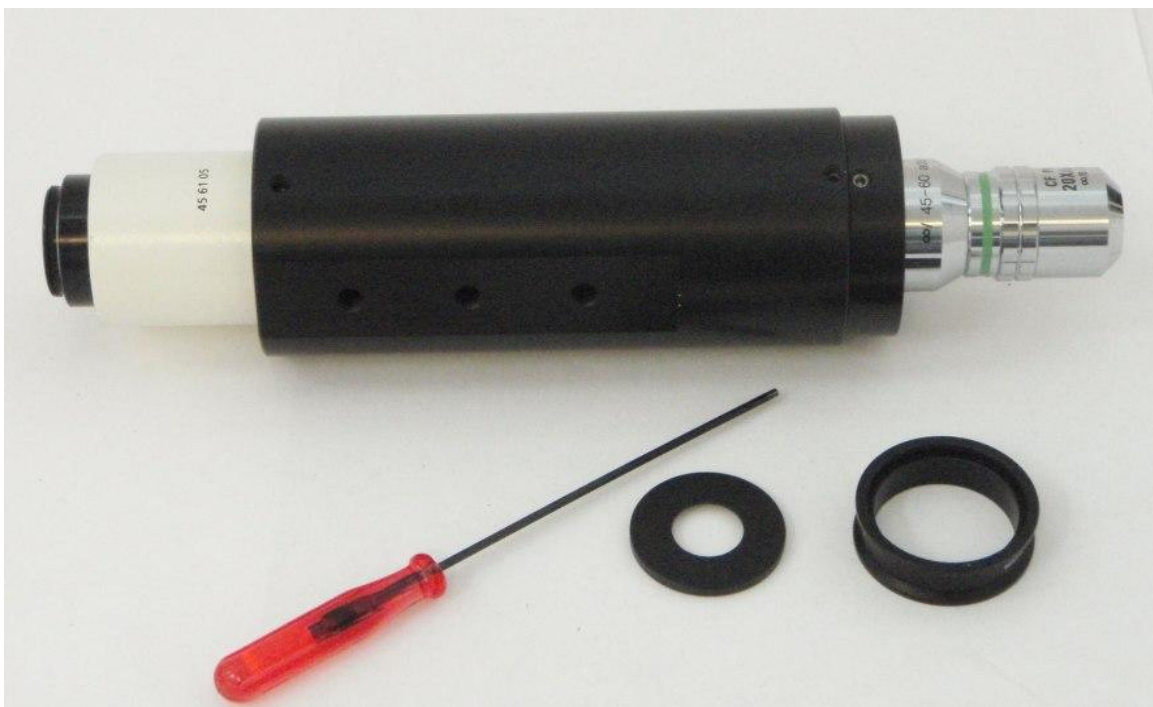
Figure 1: Simplest microscope configuration has C-mount for camera, tube with a tube lens, and an objective lens. Coupling ring connects modules; stop ring can be placed wherever there is a coupling ring. The 2 mm Allen driver is the main assembly tool.
