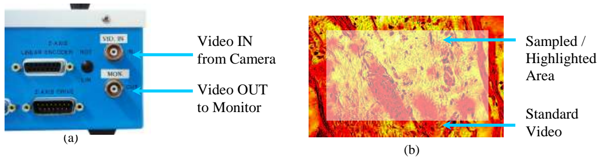
Fig 1: (a) Relevant Auto-focus Connections (b) Screenshot of Video Monitor signal from the Auto-Focus controller showing Sampled/Highlighted Area
