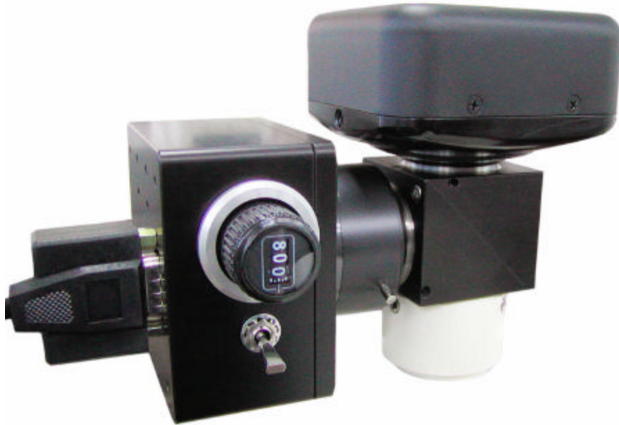
PhotoTrack Sensor Module and a Digital Camera mounted to a Beam Splitter
