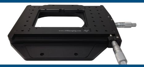
The MIC-2500 Manual Stage is a specifically designed, precise, stable platform for piezo scanning stages and comes standard with manual micrometers. The MIC-2500's standard configurations flat top plate allows for mounting XYZ piezo stages, manual manipulators, and uses ASI's K size inserts.
