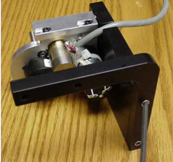
Attach roll back plate to motor drive
