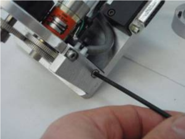
Figure 5b Loosen, but do not remove vertical adjustment screws
