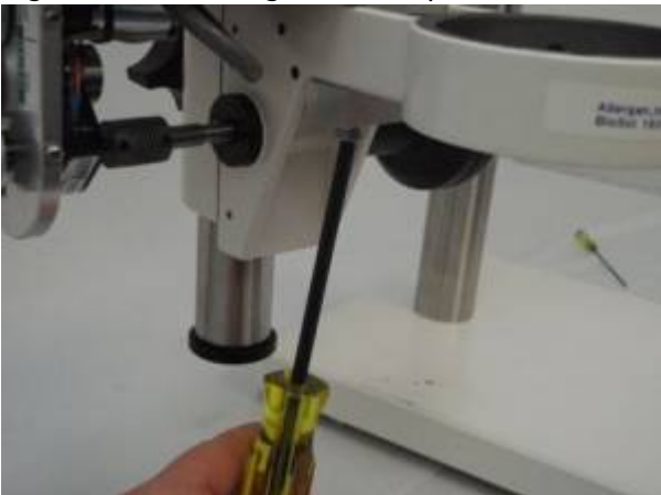
Figure 7c Mounting the base plate.
