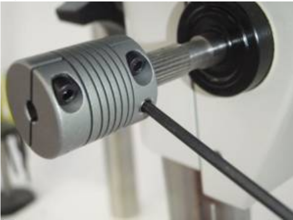
Figure 4c. Installing Helix coupler onto focus shaft.
