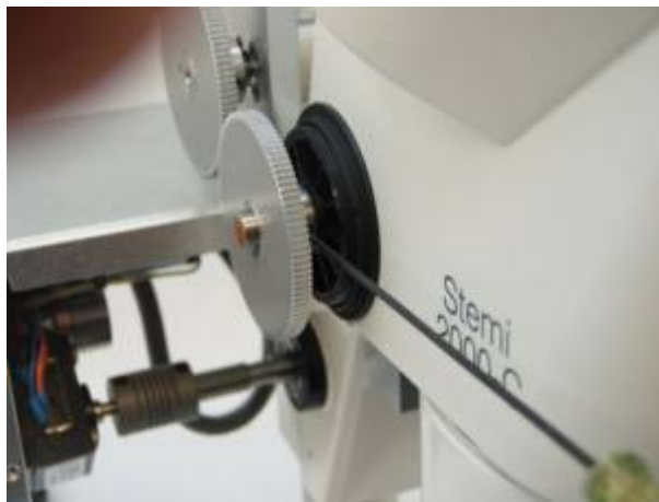
Figure 11b. Align gears as shown
