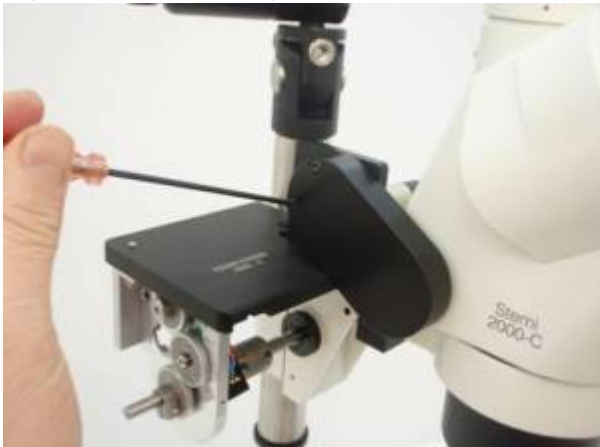
Figure 12c. Installing the zoom drive cover
