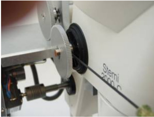
Figure 11b. Align gears as shown
