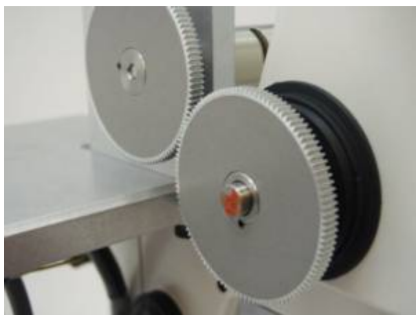
Figure 11a. Align gears as shown
