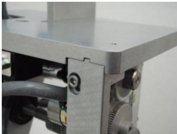
Figure 8d. Installing the Z drive.
