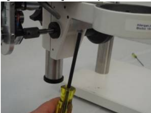
Figure 7c Mounting the base plate.
