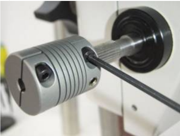
Figure 4b. Installing Helix coupler onto focus shaft.
