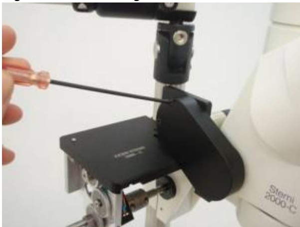
Figure 12b. Installing the zoom drive cover
