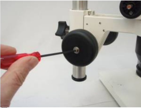
Figure 1a remove left fine focus knob
