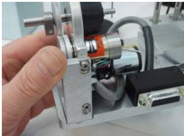
Figure 5a Loosen, but do not remove vertical adjustment screws
