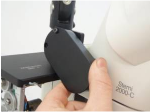
Figure 12a. Installing the zoom drive cover
