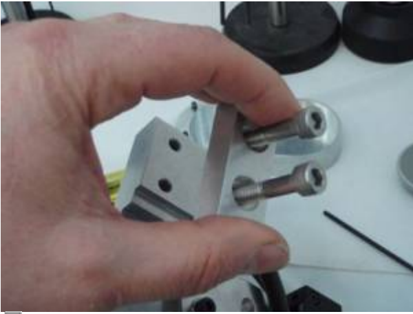
Figure 7a Mounting the base plate.
