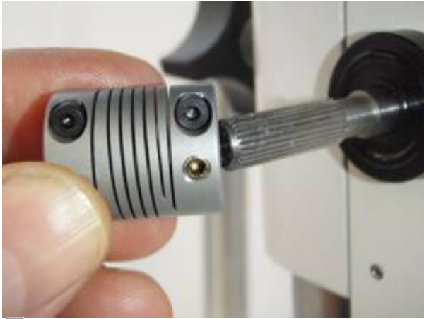
Figure 4a. Installing Helix coupler onto focus shaft.
