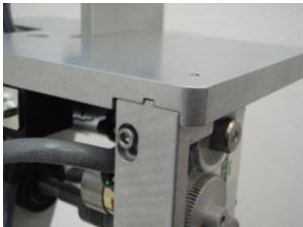
Figure 8d. Installing the Z drive.
