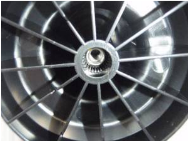
Figure 1c remove left fine focus knob
