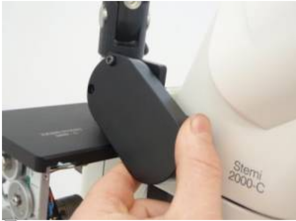
Figure 12a. Installing the zoom drive cover
