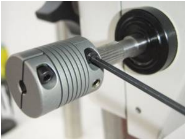
Figure 4b. Installing Helix coupler onto focus shaft.
