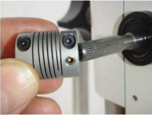
Figure 4a. Installing Helix coupler onto focus shaft.
