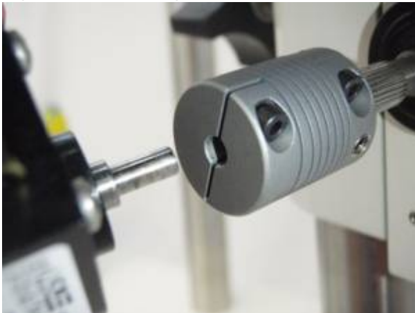
Figure 8b. Installing the Z drive.
