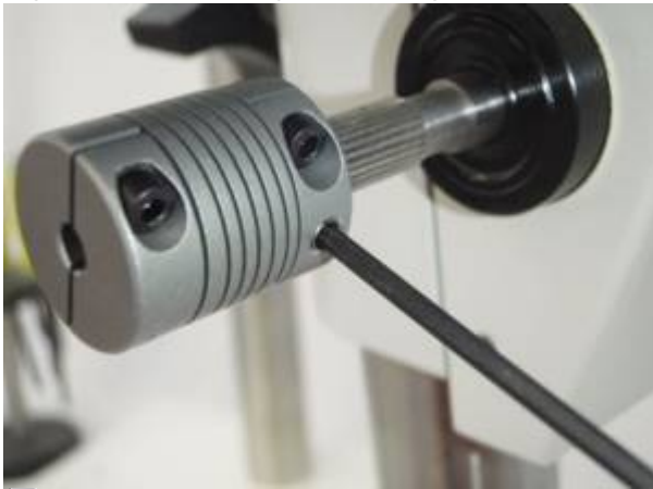
Figure 4c. Installing Helix coupler onto focus shaft.
