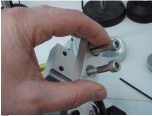
Figure 7a Mounting the base plate.
