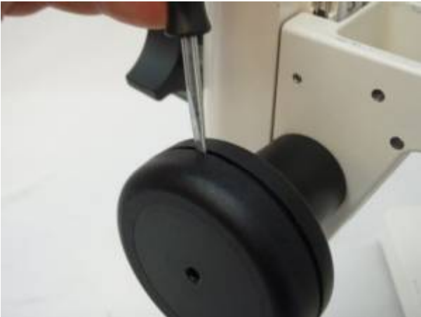
Figure 1b remove left fine focus knob
