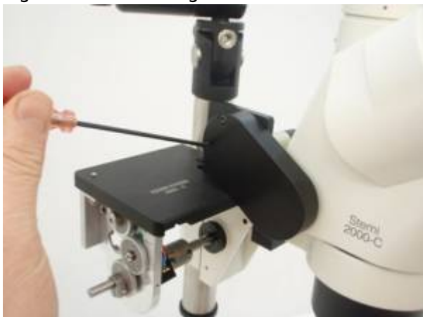
Figure 12c. Installing the zoom drive cover
