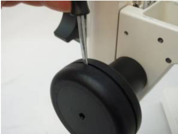
Figure 1b remove left fine focus knob
