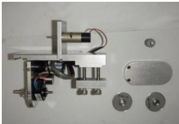
Figure 2. Z drive & Zoom components
