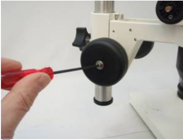
Figure 1a remove left fine focus knob
