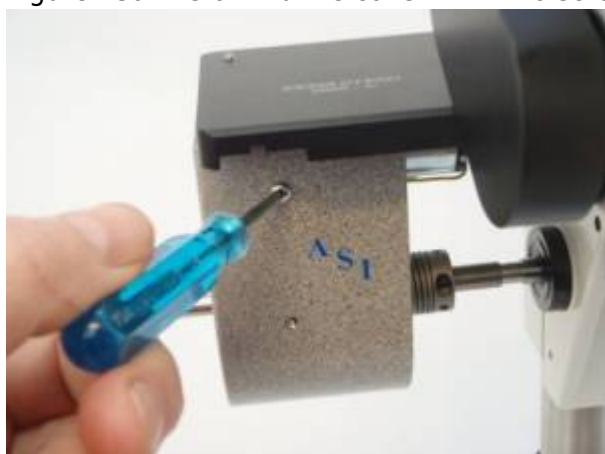
Figure 13b. Install Z drive cover with two screws provided
