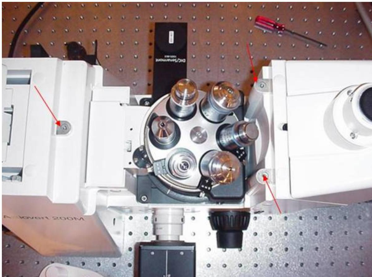
Location of three 4 x 12 mm screws that secure stage to Axiovert /AxioObserver. There are two in the front & one in rear. Use 3mm Allen wrench to remove screws & then remove stage.
