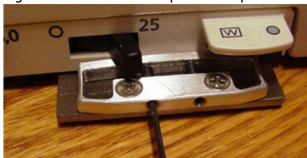
Figure 8: Install the baseplate clamp between the switches.
