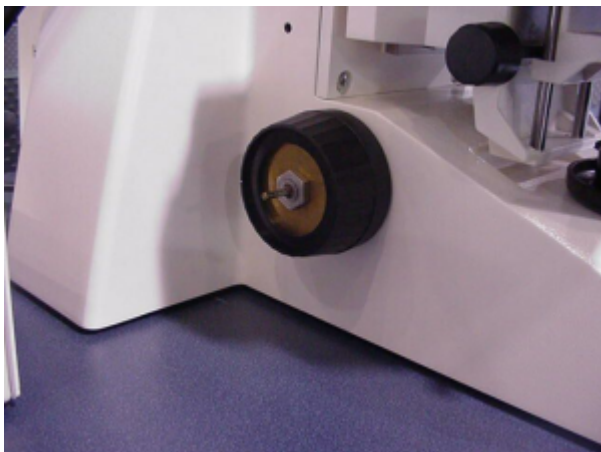
Figure 1: Fine focus knob removed
