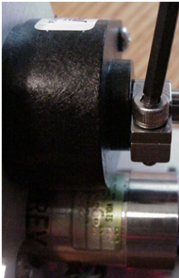
Figure 7: Tightening the drive shaft clamp.
