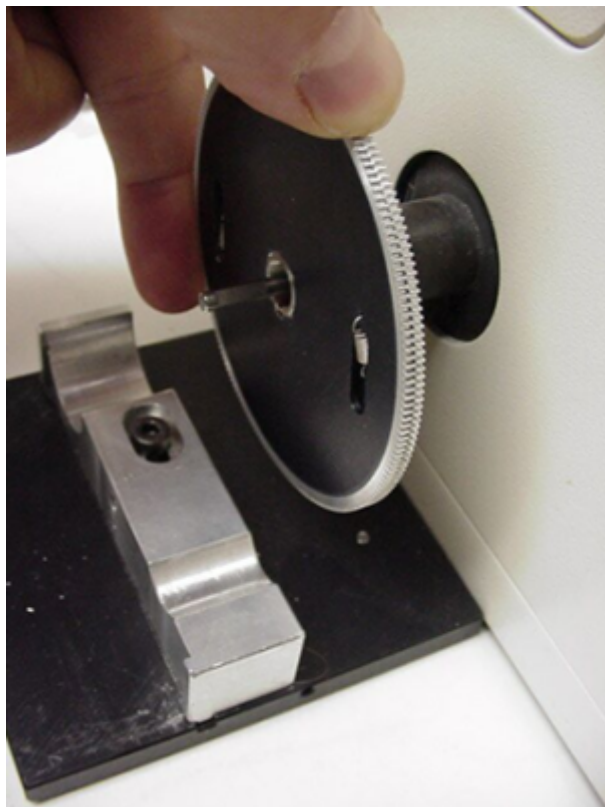
Installing Anti-Backlash gear
