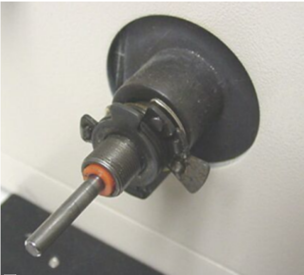
Coarse & Fine Focus Knob removed
