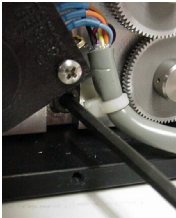
Removing the vertical adjustment screw
