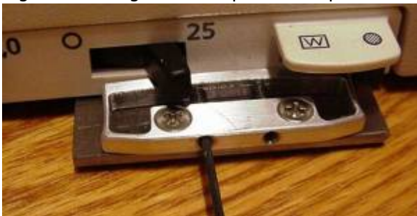
Figure 10b: Tighten baseplate clamp after drive is installed & roughly aligned
