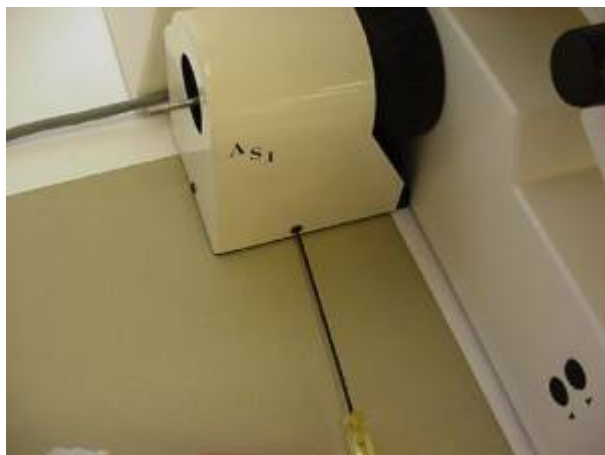
Figure 11a: Installing the cover
