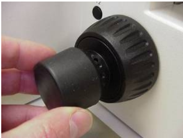
Figure 1a: Remove rubber boot
