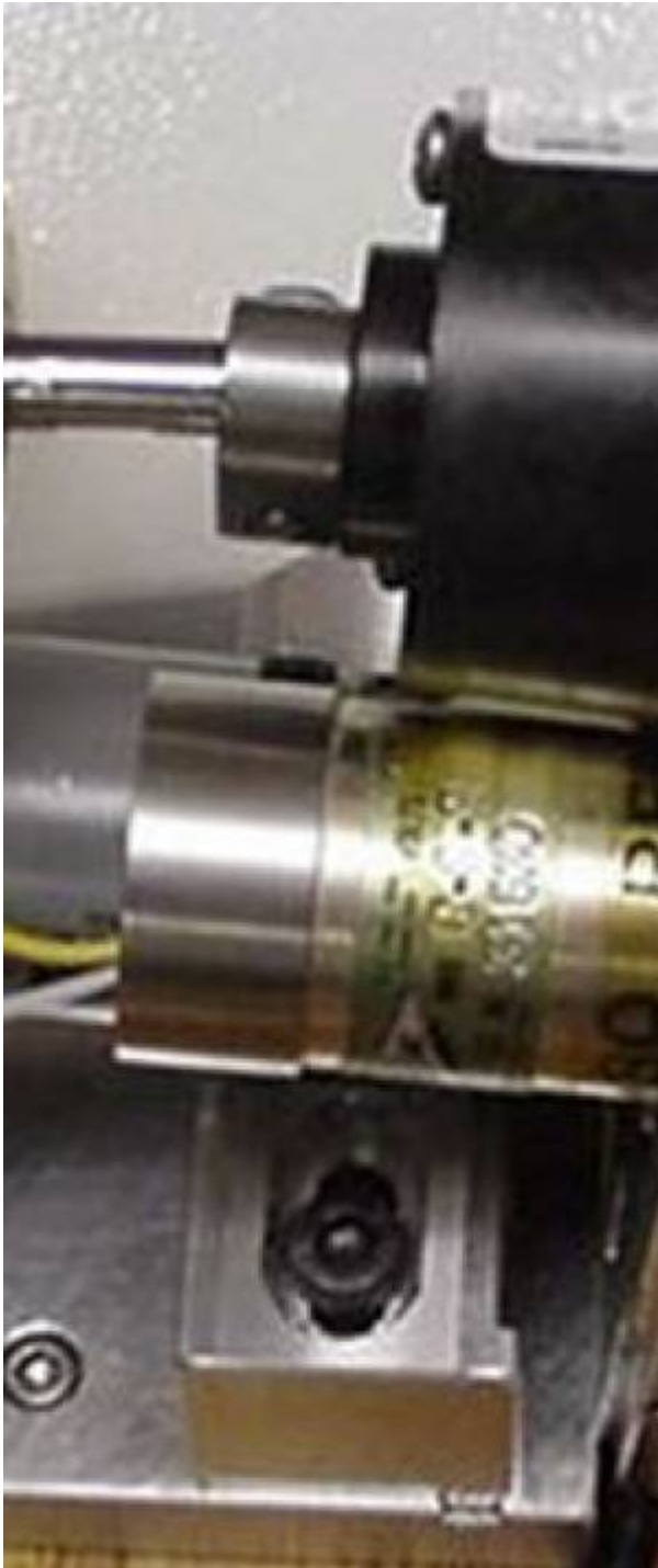
Figure 7: Slide ASI drive shaft onto microscope's fine focus shaft
