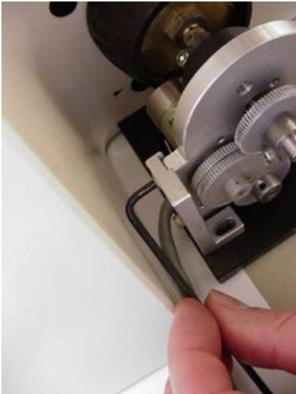
Figure 11a: Tightening the vertical & horizontal adjustment screws
