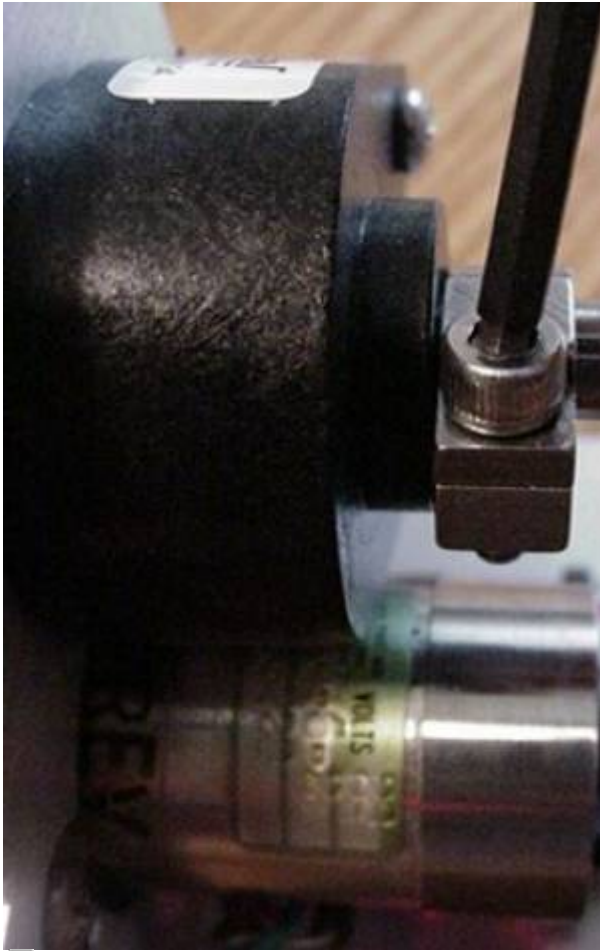
Figure 9b: Tightening the drive shaft clamp
