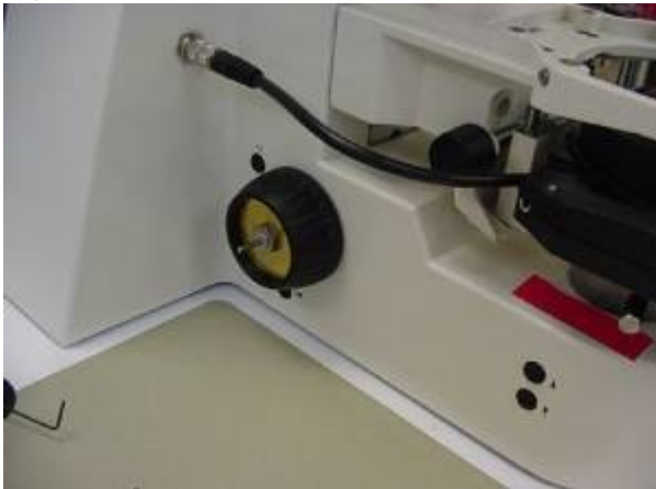
Figure 1c: Pull knob straight off to expose shaft.
