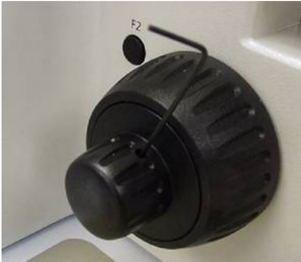
Figure 1b: Use 1.5 mm Allen wrench to loosen set screw.
