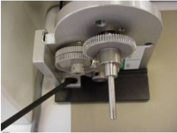
Figure 11b: Tightening the vertical & horizontal adjustment screws
