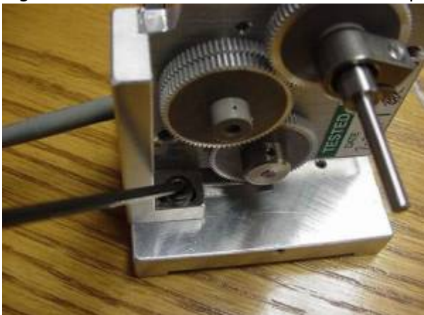
Figure 8: Install but do not tighten horizontal adjustment screw
