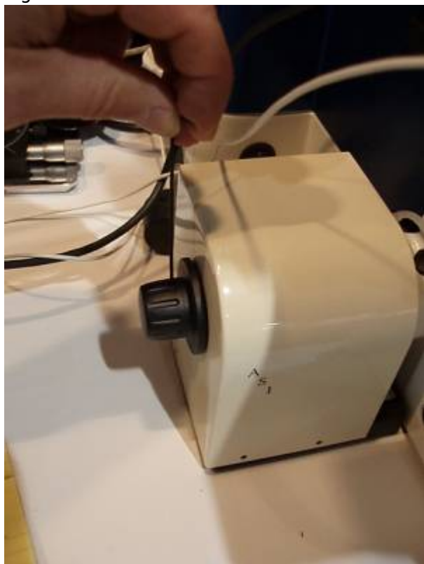
Figure 11d: Installing the cover
