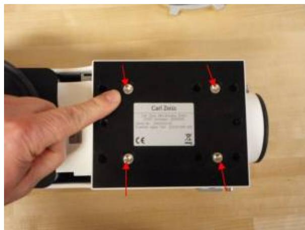
Remove top of scope as shown & then used T25 wrench to remove four screws noted that secure factory spacer
