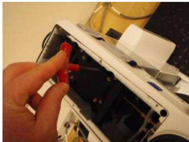
Use T25 wrench to remove small dovetail and use 3 mm wrench to remove stops and install these on longer supplied dovetail as shown below
