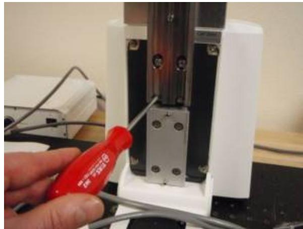
Use the original screws with fresh blue lock tight to attach the longer dovetail as shown. Attach the bottom screws first & insure the longer dovetail is aligned parallel to the bottom dovetail; this can be done by using a straight edge
