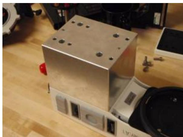
Use original screws that secured short factory spacer & T25 wrench to secure longer spacer onto top of microscope as shown in photos below.
