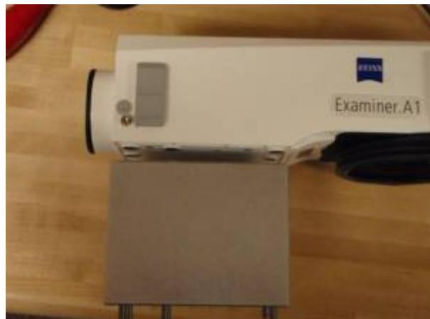
Align spacer block with top of microscope as shown above, then flip top of microscope & microscope as shown below.
