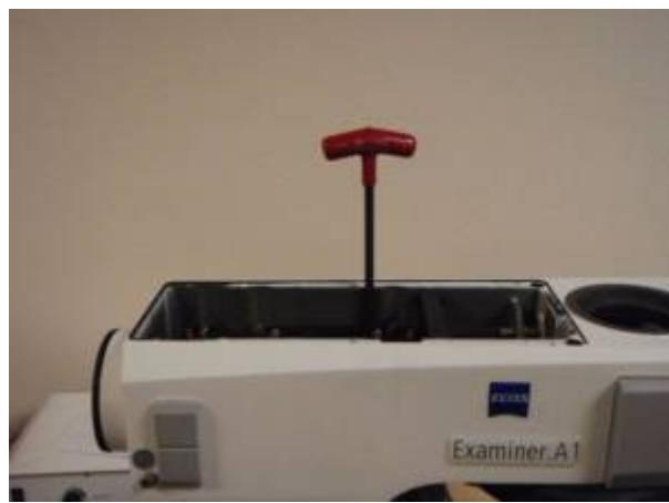
Remove the top cover as shown & loosen the six screws noted with a 5 mm Allen wrench as shown.
