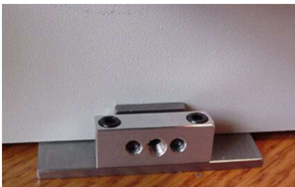
Figure 9: Tighten baseplate clamp after drive is installed & roughly aligned
