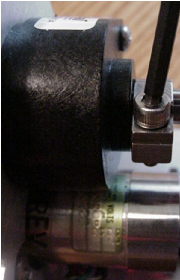
Figure 10: Tightening the drive shaft clamp
