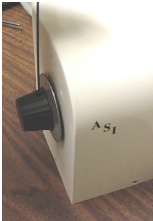
Figure 9. After the drive is properly aligned and secured install the cover as shown, and then install the fine focus knob.
