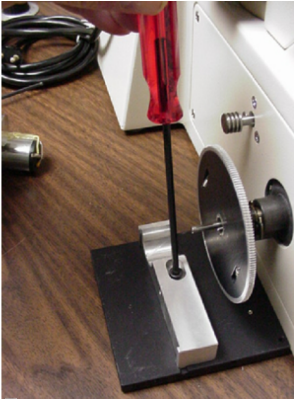
Figure 6. Use the 3mm Allen wrench to loosen the horizontal adjustment screw.
