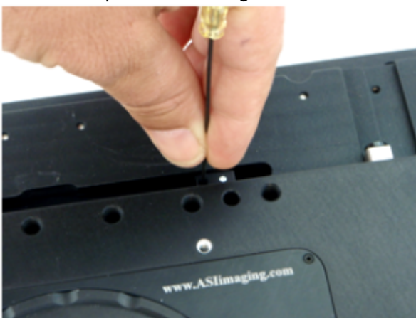
Figure 5b: After loosening the setscrew as shown in figure 2a, move the limit until the “L” appears in the X-axis display as shown in figure 6c. Do not over-tighten.
