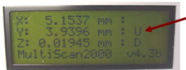
Figure 4c Upper limit U displayed on Y-axis
