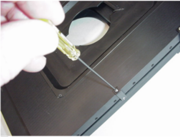
Figure 5b. After loosening the setscrew as shown in figure 2a, move the limit until the "L" appears in the X-axis display as shown in figure 5c. Do not over-tighten.
