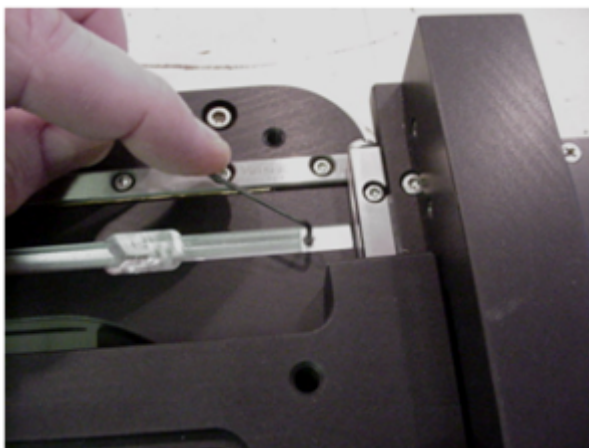
Figure 2a. Loosening setscrew so that you can move the X-axis lower limit switch sensor. Do not Over-tighten
