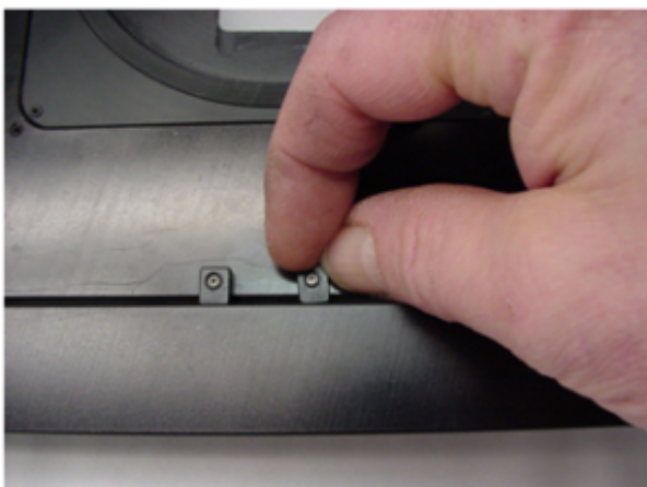
Figure 5b. After loosening the setscrew as shown in figure 2a, move the limit until the “L” appears in the X-axis display as shown in figure 5c. Do not over-tighten.
