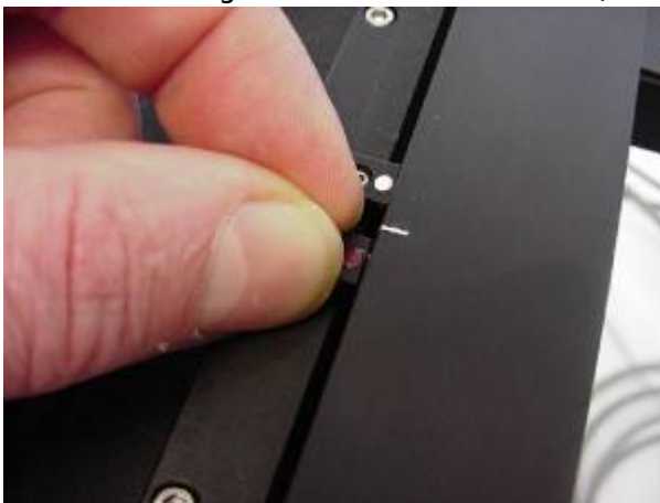
Figure 4b. After loosening setscrew as shown in figure1b. Move the sensor until the U appears in the Y-axis display as shown in figure 4c. Do not over-tighten
