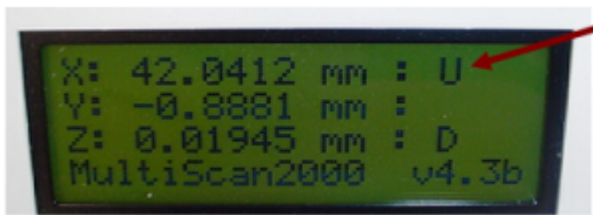
Figure 6c. Upper limit U displayed on X-axis
