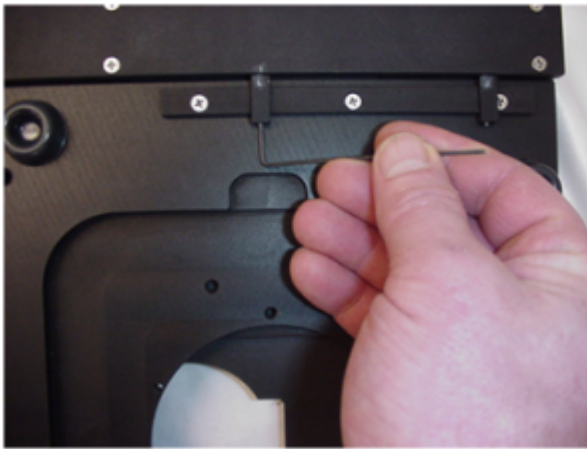
Figure 2a. Loosen the setscrew so that you can move the X-axis lower limit located at the bottom left front of the stage. Do not over-tighten.
