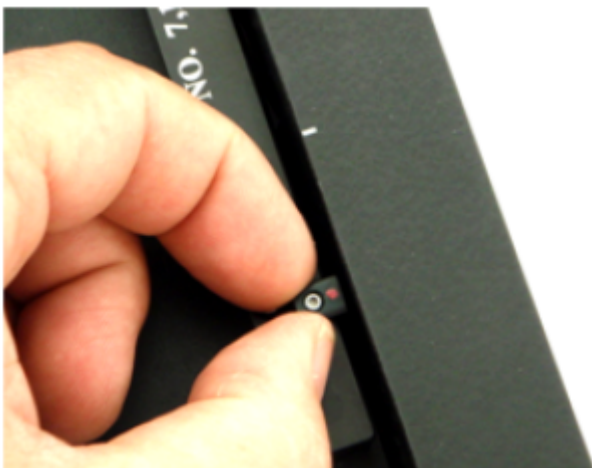
Figure 4b: After loosening the setscrew as shown in figure 1b, move the limit until the “U” appears in the Y axis display as shown in figure 4c. Do not over-tighten.
