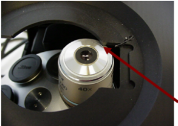
Figure 3a. Move stage in Y-axis so that it almost hits objective as shown
