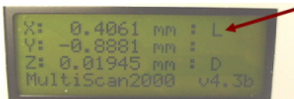
Figure 5c. Lower limit L displayed on X-axis
