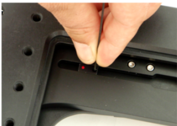
Figure 6b: After loosening setscrew as shown in figure 2b, move the limit until the “U” appears in the X-axis display as shown in figure 7c. Do not over-tighten.
