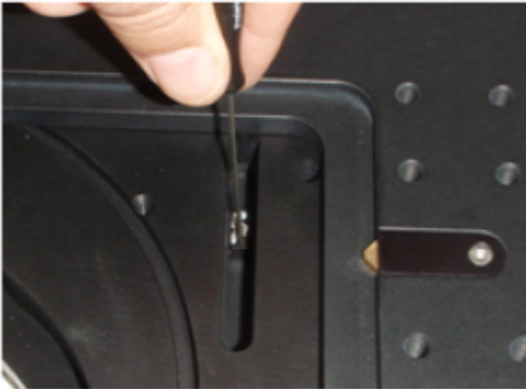
Figure 2a. Loosen the setscrew so that you can move the Y-axis lower limit located at the top right of the stage. Do not over-tighten.
