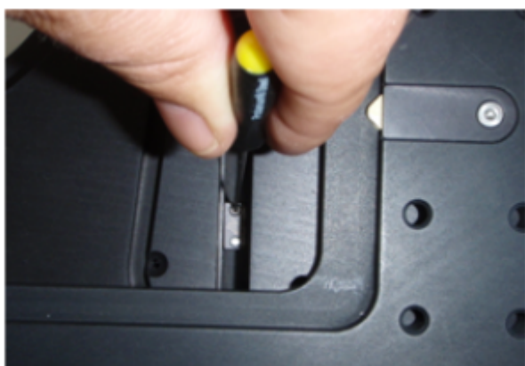
Figure 4b. After loosening the setscrew as shown in figure 2b, move the limit until the “U” appears in the Y axis display as shown in figure 4c. Tighten the set screw. Do not over-tighten.
