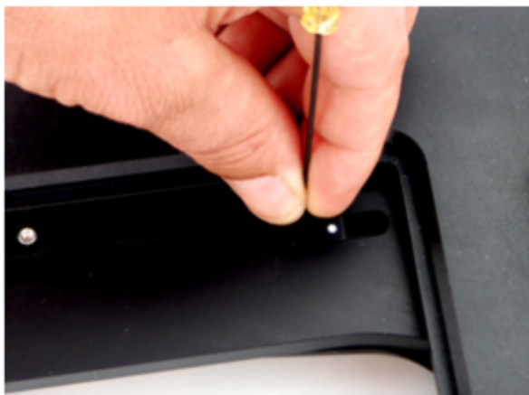
Figure 5b: After loosening the setscrew as shown in figure 2a, move the limit until the “L” appears in the X-axis display as shown in figure 6c. Do not over-tighten.
