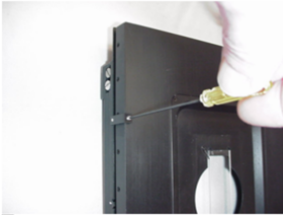
Figure 1a. Loosen the setscrew so that you can move the X-axis lower limit located at the front left of stage. Do not over-tighten.
