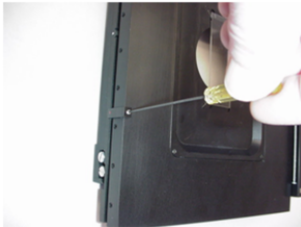
Figure 1b. Loosen the setscrew so that you can move the X-axis upper limit located at the rear left of stage. Do not over-tighten.
