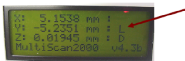
Figure 3c. Lower limit L displayed on Y-axis
