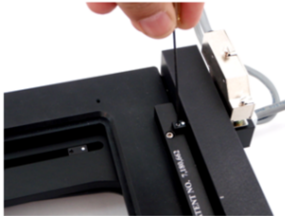
Figure 1a: Loosen the setscrew so that you can move the Y-axis lower limit located at the rear right of stage. Do not over-tighten.
