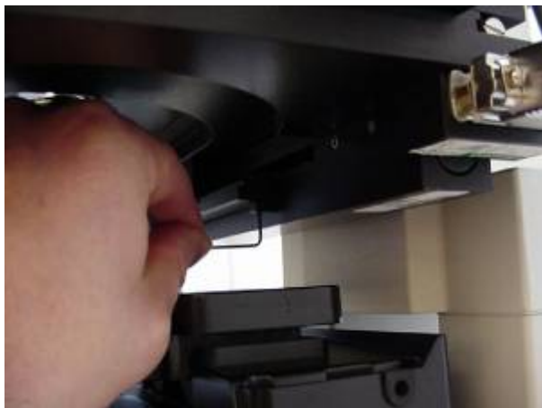
Figure 2a: Loosen the setscrew so that you can move the X-axis lower limit located at the right rear of the middle plate of stage. Do not over-tighten.
