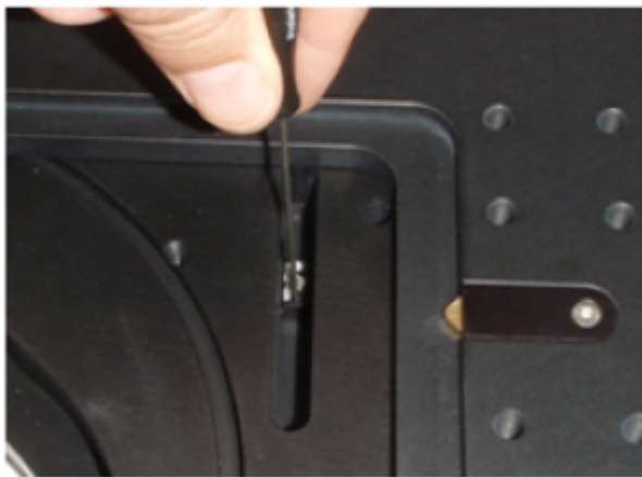
Figure 3b. After loosening the setscrew as shown in figure 2a move the limit until the “L” appears in the Y axis display as shown in figure 3c. Tighten the set screw. Do not over-tighten.
