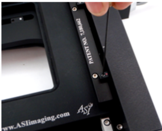
Figure 1b: Loosen the setscrew so that you can move the Y-axis upper limit located at the front right of stage. Do not over-tighten.
