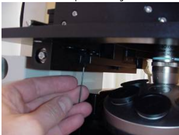
Figure 2b: Loosen the setscrew so that you can move the X-axis upper limit located at the left rear of the middle plate of stage. Do not over-tighten.
