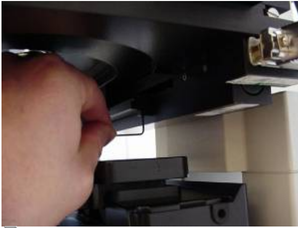
Figure 2a. Loosen the setscrew so that you can move the Y-axis lower limit located at the bottom right rear of the stage. Do not over-tighten.
