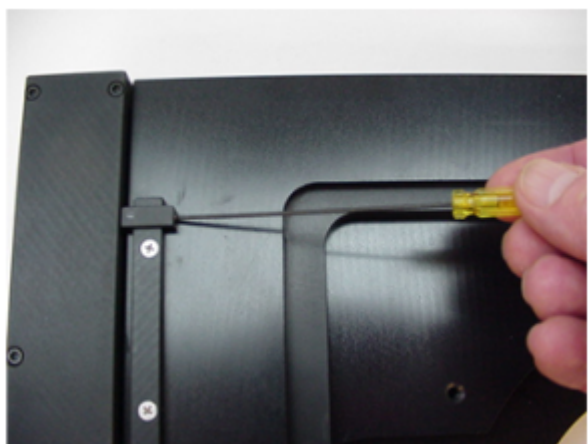
Figure 1b. Loosen the setscrew so that you can move the Y-axis upper limit located at the rear left of stage. Do not over-tighten.
