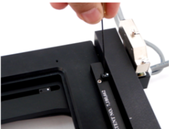
Figure 1a: Loosen the setscrew so that you can move the Y-axis lower limit located at the rear right of stage. Do not over-tighten.
