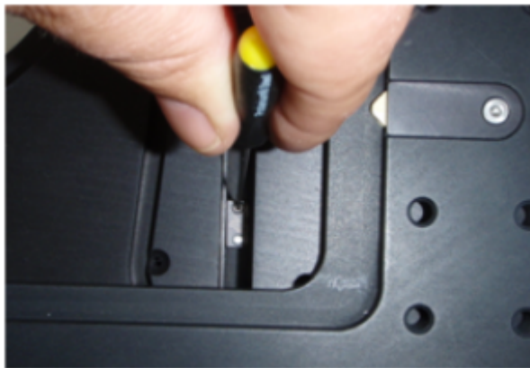
Figure 2b. Loosen the setscrew so that you can move the Y-axis upper limit located at the bottom right of the stage. Do not over-tighten.
