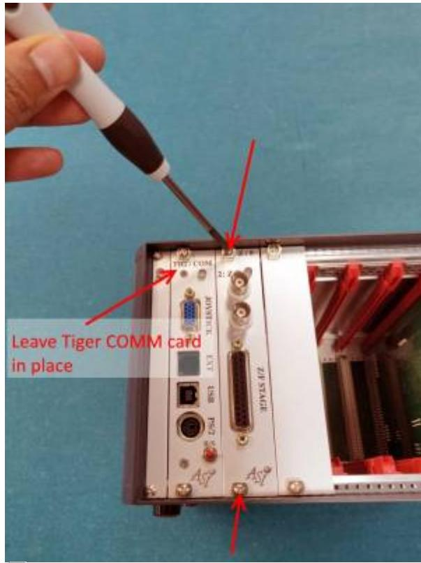
Use a flat screwdriver to unscrew the two screws holding the card in place
