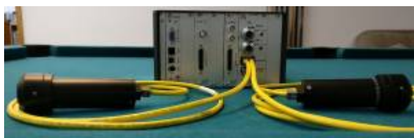
TGPMT card shown connected to two PMTs
