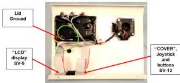
STEP 6: Next, check to see that all the wires are routed away from the joystick and that the case is clean and clear of foreign debris, (screws, washers, etc.). The lid can now be screwed back on with the six 4-40 screws in reverse order of step 2. Next, shake the case to make sure that nothing is rattling around inside the case.
