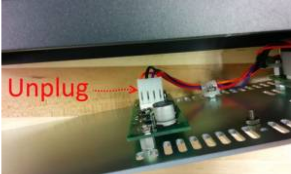
Figure 5: Unplug the Power supply connector
