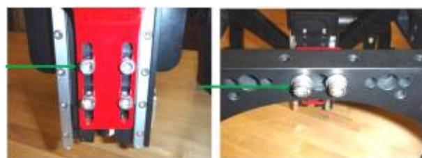
STEP 3: The bottom four screws are removed with the 5mm Allen wrench.
