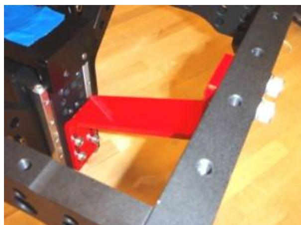
STEP 2: Locate the six cap screws that retain the bracket.
