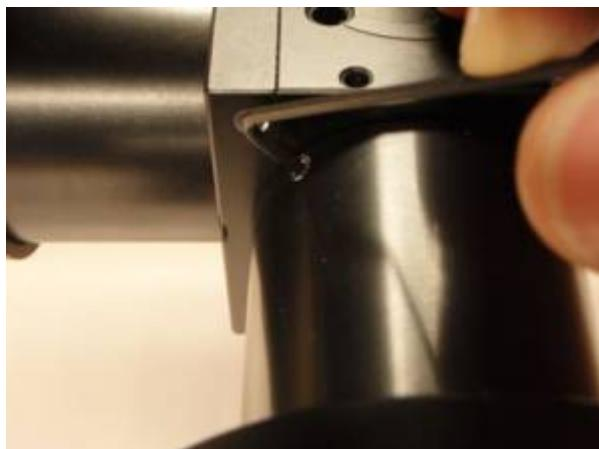
STEP 3: Remove the bottom two set screws with the 2mm socket driver.
