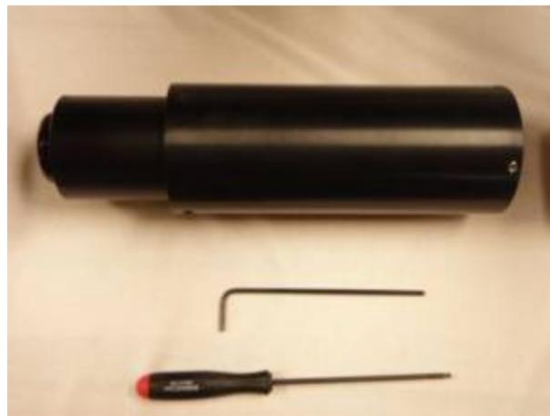
STEP 6: Pull the tube out of the tube clamp pair. Tape or bag the tubes optical ends as well as the optical path of the RAMM to keep dust out of the light train. If the RING "A" needs to be removed there are three set screws that must also be removed. Now you are ready to add a new tube to the RAMM. Follow these directions in reverse to mount the tube.
