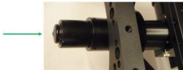
STEP 2: Remove the top two metric set screws with the 2mm Allen wrench.
