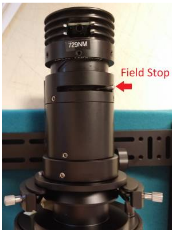
Fig. 1 The field stop iris is located just below the LED housing.
