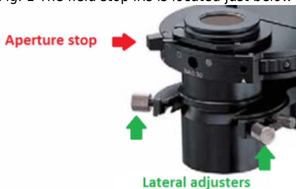
Fig. 2 The aperture stop changes the brightness and illumination NA. Lateral adjusters center the field stop on the camera sensor.
