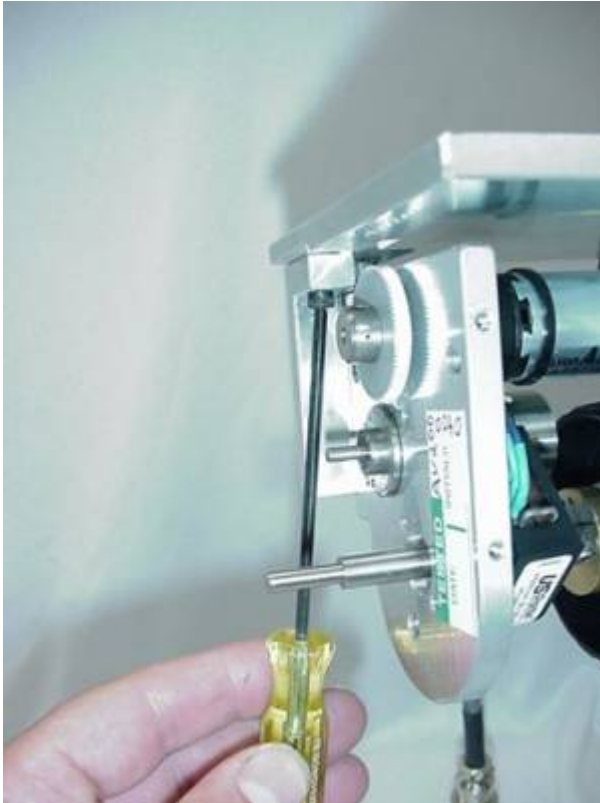
Figure 8. Align drive and install horizontal adjustment screw
