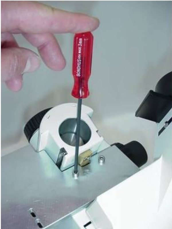
Figure 5. Use the two 5x 10 mm socket head cap screws to secure the baseplate to the microscope
