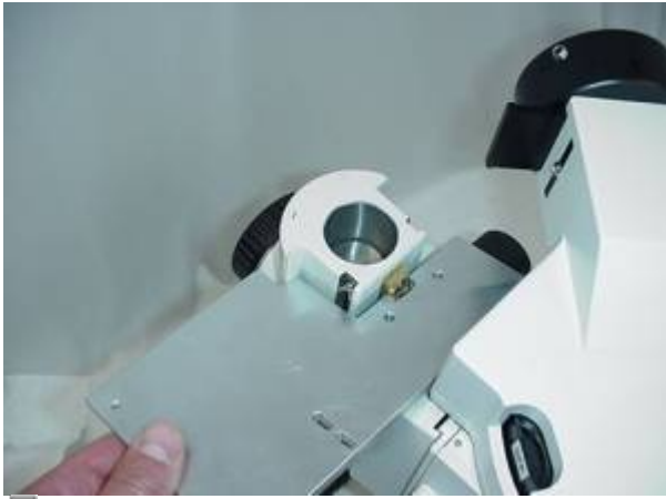
Figure 4 Use existing holes on microscope to mount base plate as shown
