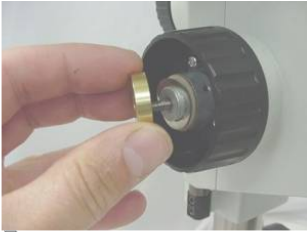
Figure 6b. Install clutch plate as shown
