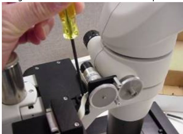
Figure 15. When gears are properly aligned use the 7/64" Allen wrench to tighten the screw that secures the zoom motor.
