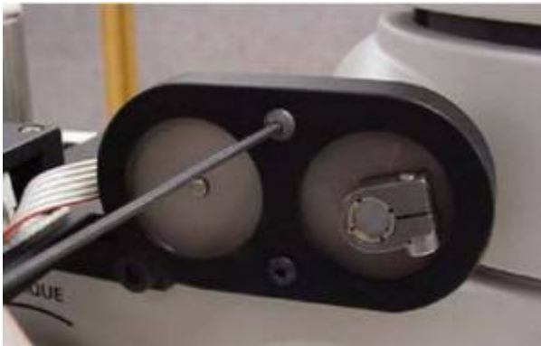
Figure 17. Check the alignment by noting the drag while turning the right zoom knob. No noticeable drag should be felt at any point with in the full 360 degrees of rotation. If any noticeable drag is felt loosen the Zoom assembly and realign it. If alignment is correct use the 1/16" Allen wrench to install the cover as shown .
