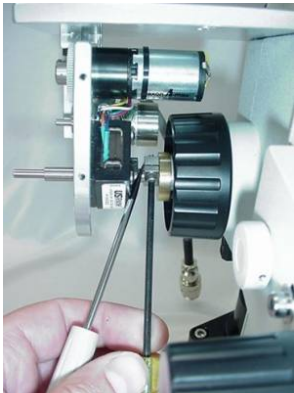
Figure 9. Use a screwdriver to push the drive clamp up against clutch plate & tighten
