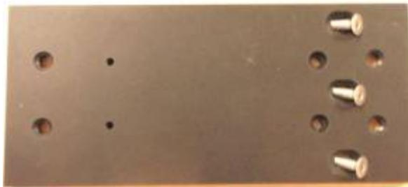
Second, remove the microscope head from the ring mount and screw the ring mount to the adapter plate with the provided three screws.
