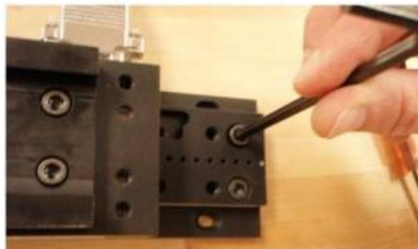
Fifth, move the LS-50 to the lower position to expose the last two mounting holes. Attach the microscope ring mount and adapter plate to the LS-50 with the last two provided screws.
