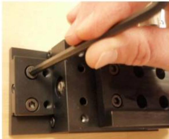
Fourth, move the LS-50 by the controller to the upper position to expose the first two mounting holes. Attach the microscope ring mount and adapter plate to the LS-50 with the provided screws.
