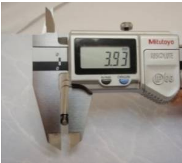
Threaded diameter of ASI's 4 mm drive shaft
