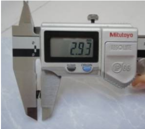
Threaded diameter of ASI's 3 mm drive shaft
