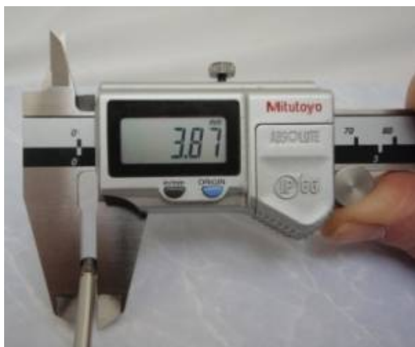
Typical diameter of threaded end of Olympus 4 mm fine focus shaft
