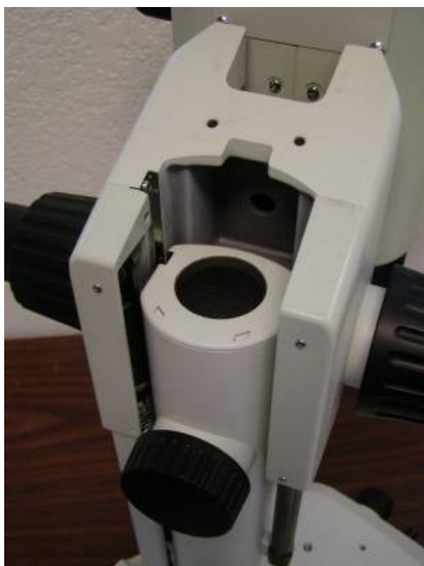
Figure 4. The focus assembly will rise up, or fall depending upon the load, when the ffk is removed.
