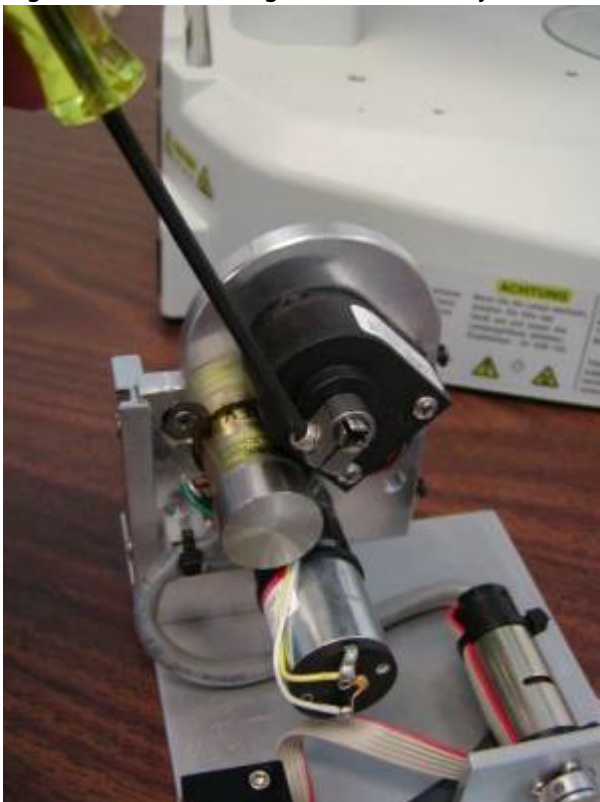
Figure 13. Loosening the drive shaft clamp
