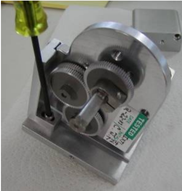
Figure 11. Loosen & remove the horizontal adjustment screw
