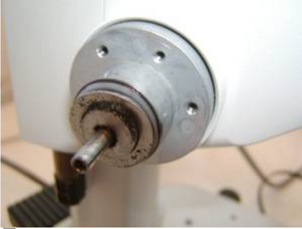
Figure 6. Use a cross blade screwdriver to loosen the three Philip head screws and remove the coarse focus knob as shown.
