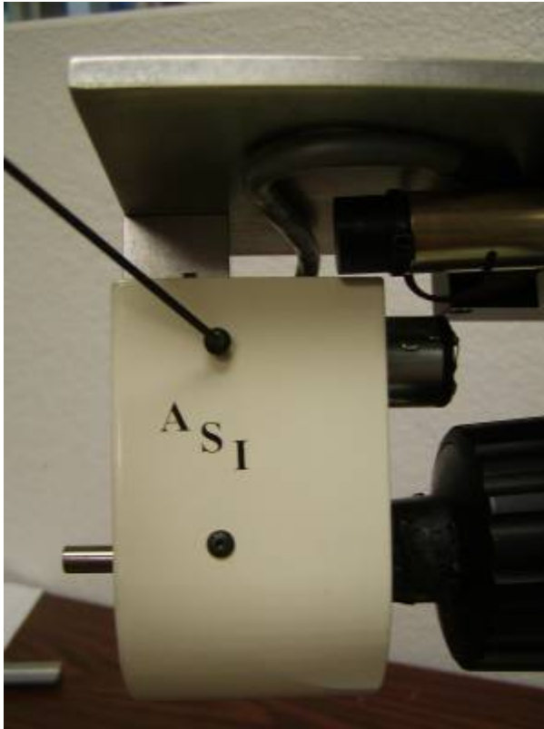
Figure 27. Use the 1/16" Allen wrench to install the drive cover as shown.
