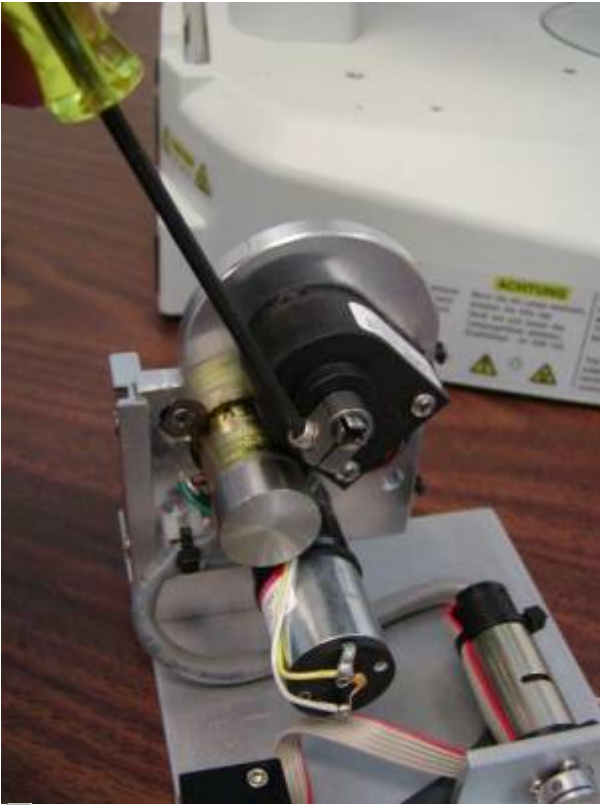
Figure 13. Loosening the drive shaft clamp
