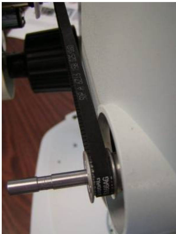
Figure 23. Location of zoom drive gear and belt. Belt is ~ 3 mm ( 1/8 inch ) away from scope body as shown.
