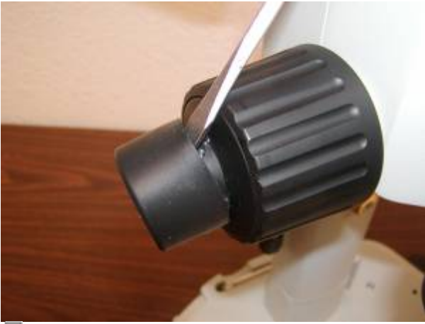
Figure 2 remove the rubber boot off of the end of the left fine focus knob
