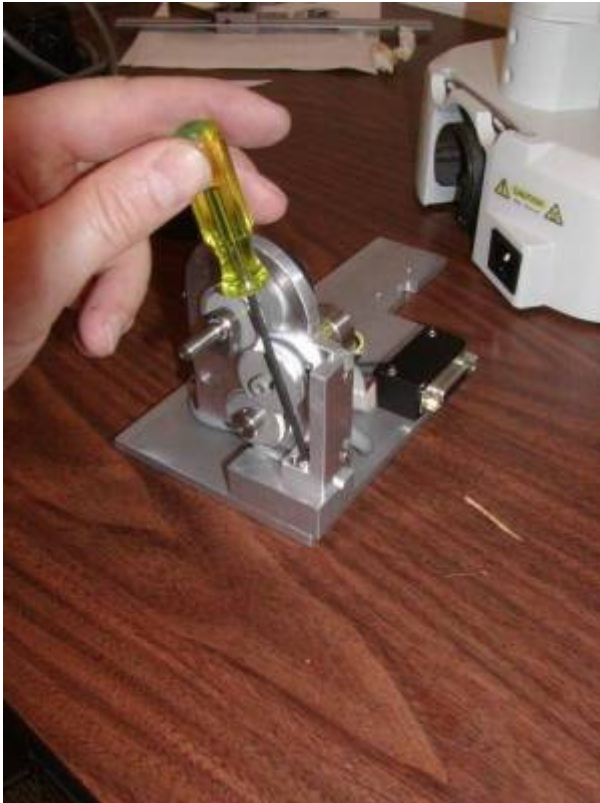
Figure 11. Loosening the horizontal adjustment screw
