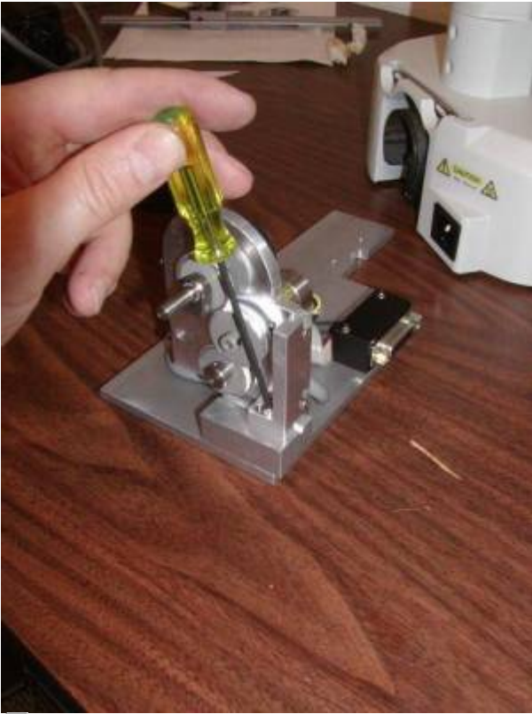
Figure 11. Loosening the horizontal adjustment screw
