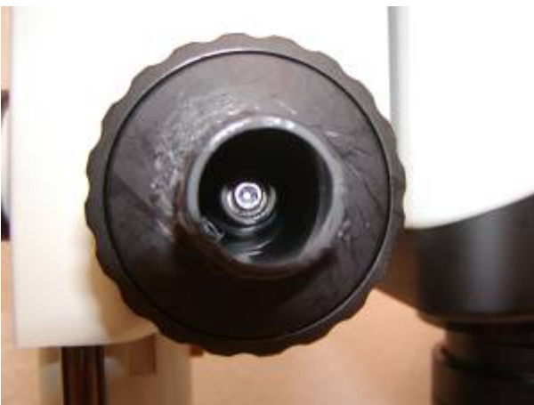
Figure 3 Location of Allen head screw to remove with 2.5 mm Allen wrench
