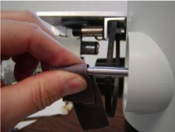
Figure 26. If you need to remove the zoom shaft belt gear you will need to sand off the slight “dings” that the zoom knob setscrews may put in the zoom shaft.
