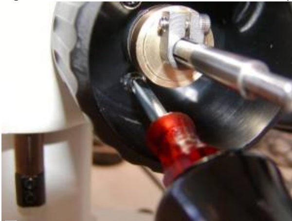
Figure 9. Install coarse knob that was removed in figure #6.
