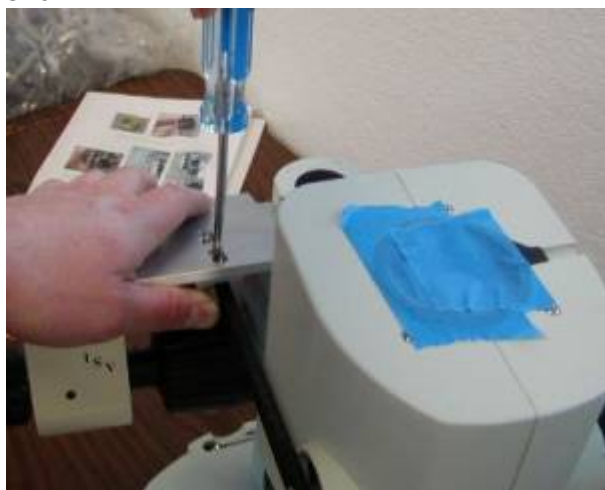
Figure 24. Push back on zoom motor assembly to tighten zoom drive belt. Use the cross blade screwdriver to tighten the two zoom motor adjustment screws.
