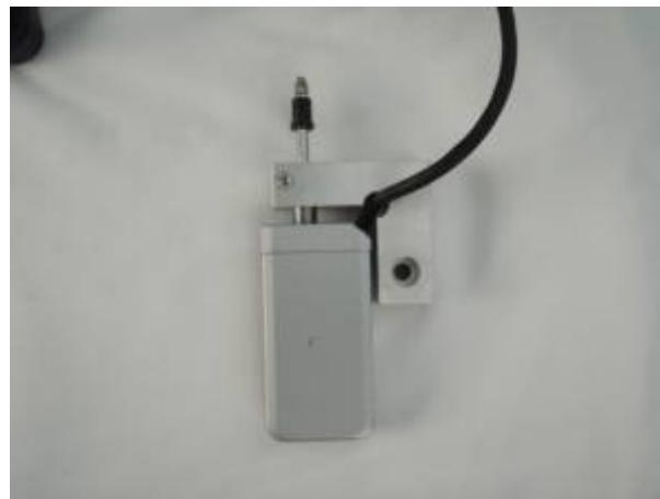
Locate the linear encoder bracket, the linear encoder, and the longer screw as shown above
