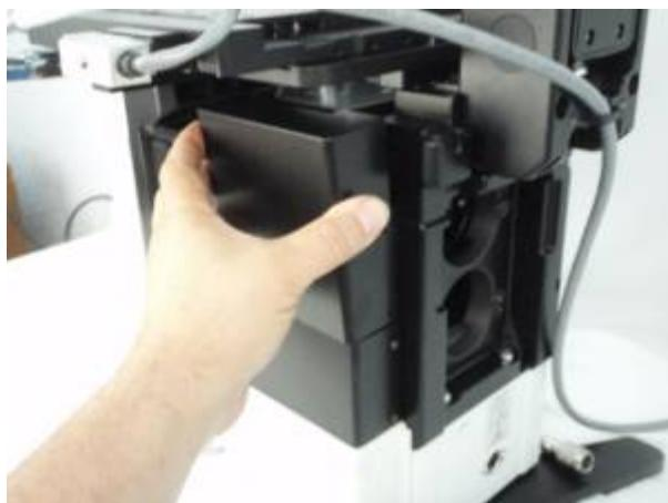
Use a medium cross screw driver to remove the two screws that secure the cover on the right side of the microscope as shown above.
