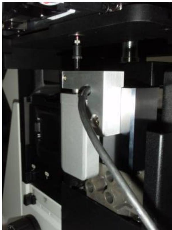
Use the Allen wrench to remove the screw as shown. Install the linear encoder bracket with the longer screw provided. Insert the linear encoder in the bracket and secure in place by tightening the screw on the bracket. Please note the end of the linear encoder will engage the stage as shown. The
