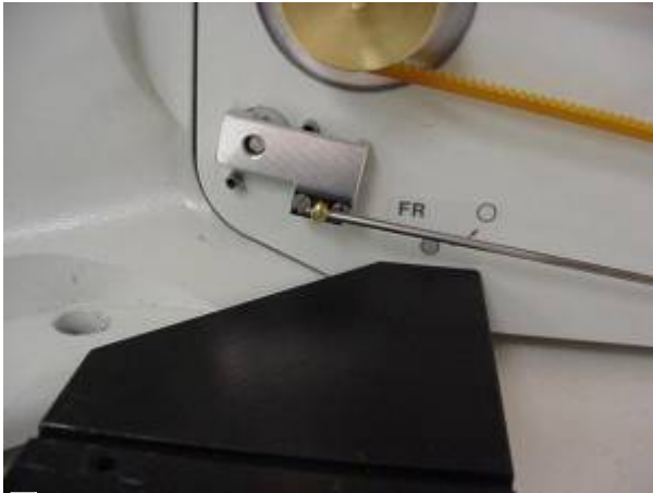
Figure 12. Diffuser switch extender with switch in second position.
