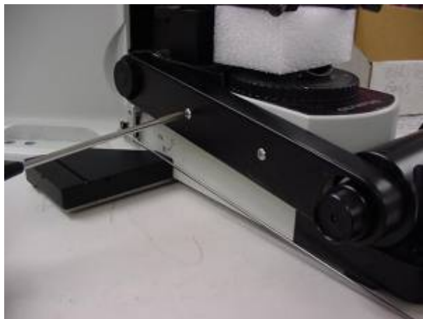
Figure 2. Use cross blade screw driver to remove belt drive cover
