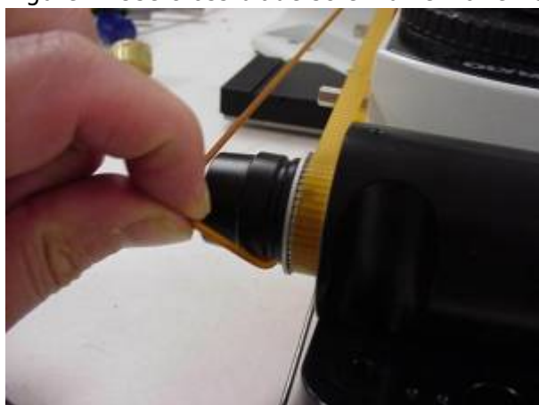
Figure 3. Remove outer drive belt
