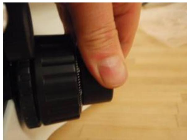
When installing the coupler insure that it is pressed all the way against the brass part of the microscope without pushing the right focus knob out at all. Check for any play in the focus shaft by pushing & pulling the right focus knob – there should be no play. Fasten the flex coupler using a 2mm Allen wrench.
