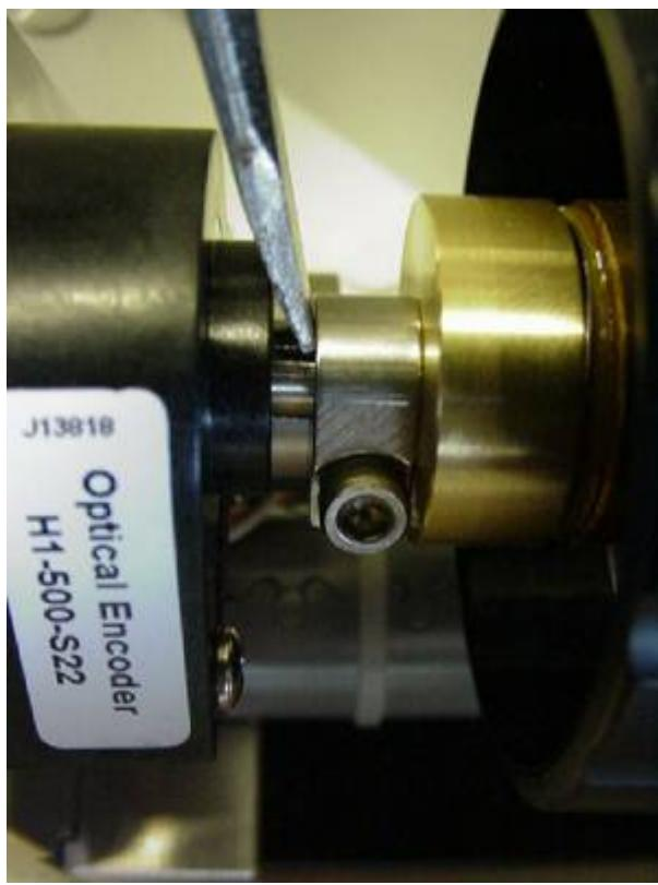
Locate the small brass clutch plate and slide it onto the fine focus shaft in place of the fine focus knob that was just removed. After the clutch plate has been installed onto the fine focus shaft install the ASI drive as outline in the next section. When tightening the clamp assembly, insure that you slide the clamp against the brass clutch plate and tighten it with the 7/64" Allen wrench as shown in the above photo.
