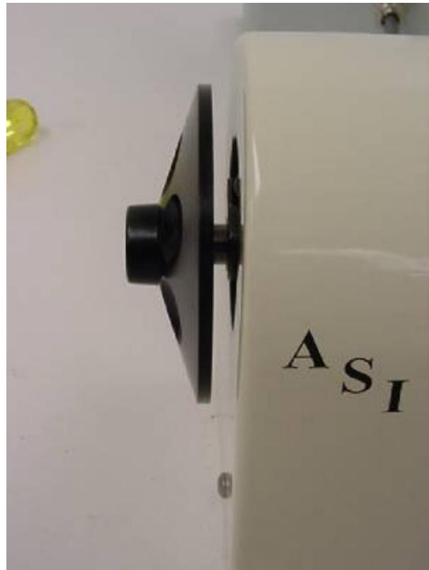
a) Locate the motor drive cover. Remove the 4/40 button head screws from the drive with the 1/16 " Allen wrench. Position the motor drive cover over the motor drive assembly and secure in place using the 4/40 button head screws.
