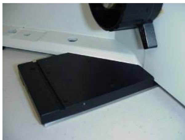
Locate the baseplate and remove the ASI drive from it if it is attached by using the Allen wrench to remove the Horizontal adjustment screw. Position the base plate assembly it so that the horizontal adjustment bar is on the left side of the microscope. Lift the front of the microscope up and slide the base plate under the microscope so that angled portion of the base plate is aligned with the contour of the microscope.
