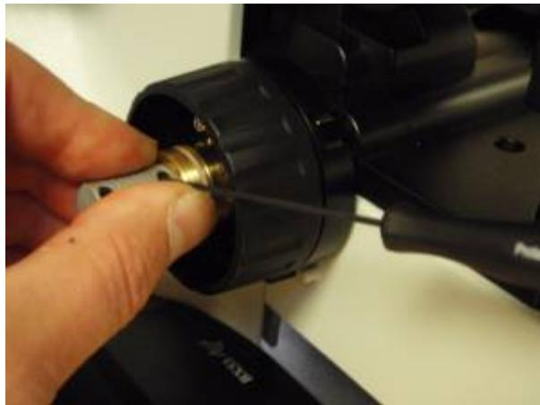
Locate the brass clutch plate and securely screw it on to the fine focus shaft. When installing the clutch insure that it is pressed all the way against the wave washer without pushing the right focus knob out at all. Check for any play in the focus shaft by pushing & pulling the right focus knob – there should be no play. Install the flex coupler as shown & fasten the flex coupler using a 1.5 mm Allen wrench.
