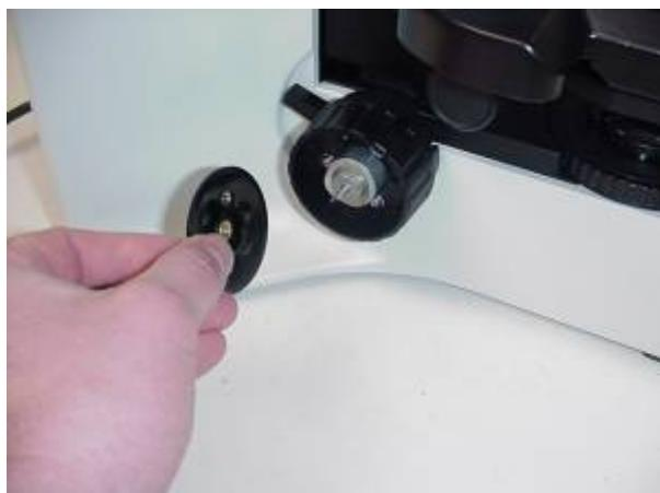
Remove the left fine focus knob from the microscope as follows:
