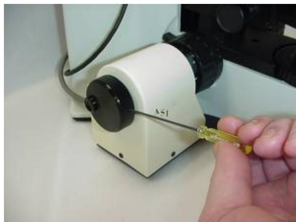
a) Locate the motor drive cover. Remove the 4/40 button head screws from the drive with the 1/16 " Allen wrench. Position the motor drive cover over the motor drive assembly and secure in place using the 4/40 button head screws.
