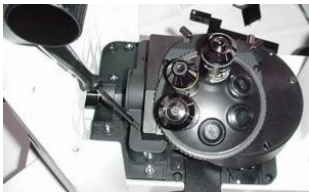
Figure 1a. Removing original screws
