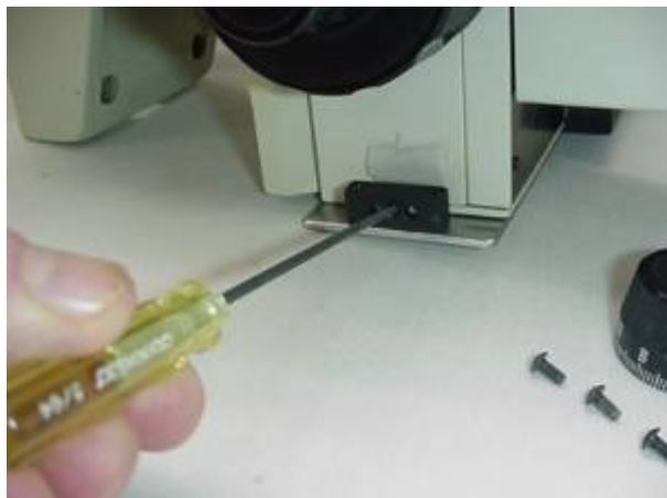
Figure 5. Use 5/64" Allen to tighten setscrew to secure clamp
