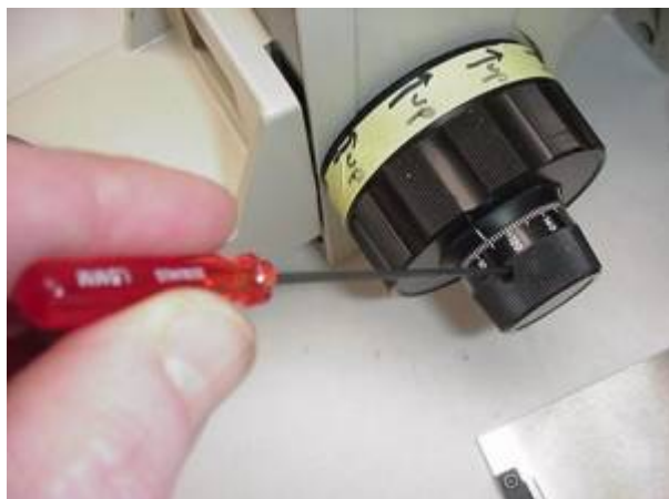
Figure 1: Use 1.5 mm Allen to loosen set screw
