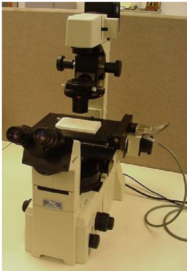
Figure 2. Stage mounted correctly with connectors & cables on the right side
