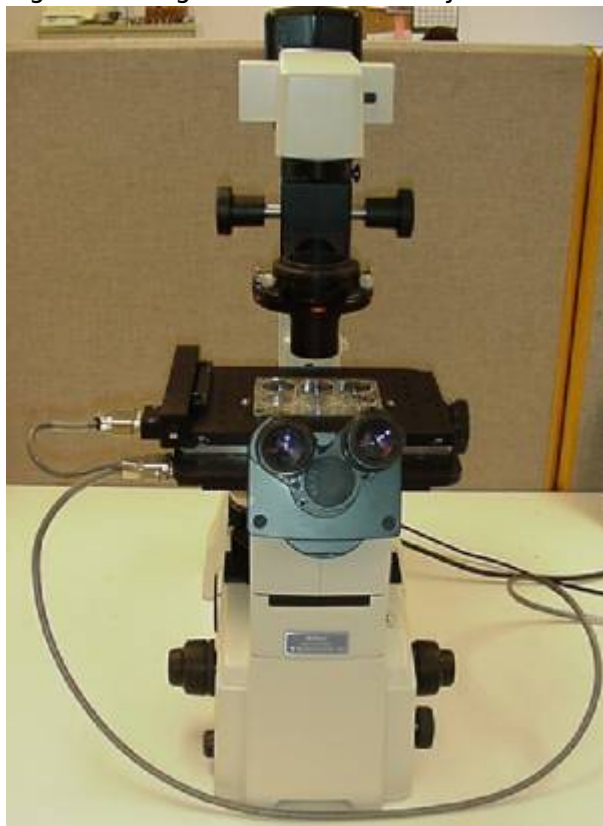
Figure 3. Stage mounted the WRONG WAY with the connectors & cables on the left side
