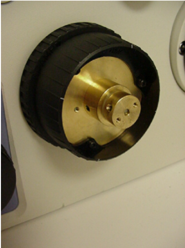
Figure 2: Pull knob straight off to expose brass adapter screws & remove brass adapter plate.
