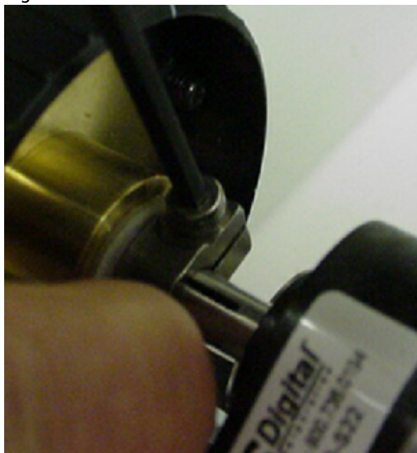
Figure 8 Press clamp against washer & tighten clamp securely to attach drive.
