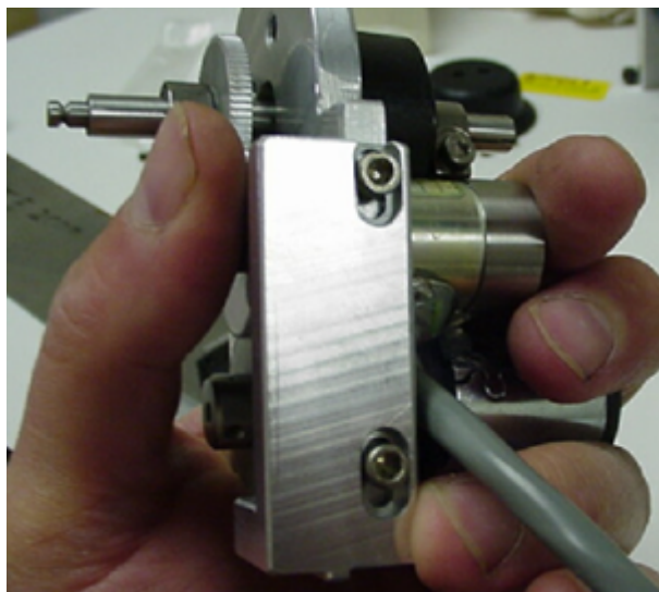
Figure 6 Loosen Vertical adjustment screws
