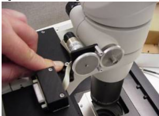
Figure 13. Loosen the screw that secures the zoom motor and press against the adjustment bar as shown so that the gears mate as shown in figure 14.
