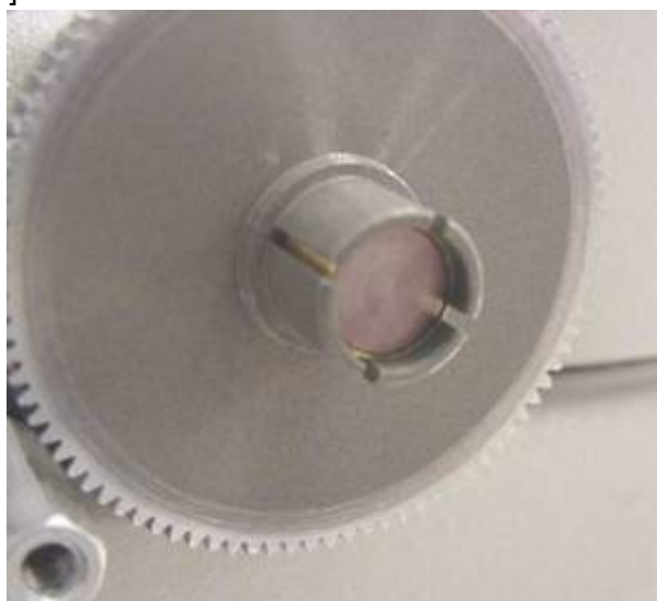
Figure 12. The zoom gear should stick out a little
