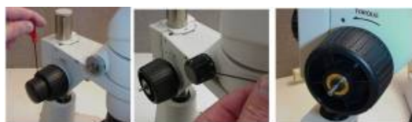
Figure 1: remove left fine focus & zoom knobs
