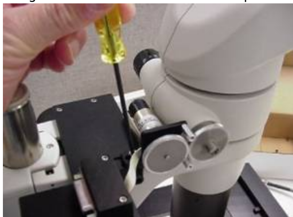
Figure 15. When gears are properly aligned use the 2.5mm Allen wrench to tighten the screw that secures the zoom motor.
