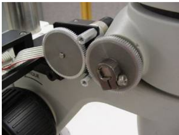
Figure 16. Install the clamp onto the zoom gear and use the 7/64" Allen wrench to tighten clamp / gear in place. Please note: clamp must be securely tightened to prevent any slippage
