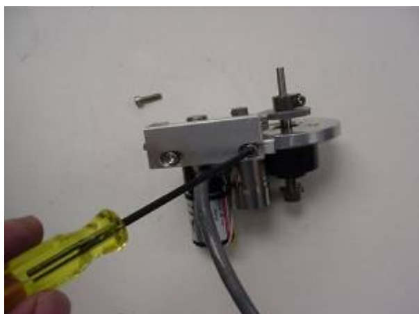
Figure 2: Z drive removed and vertical adjustment screws being loosened
