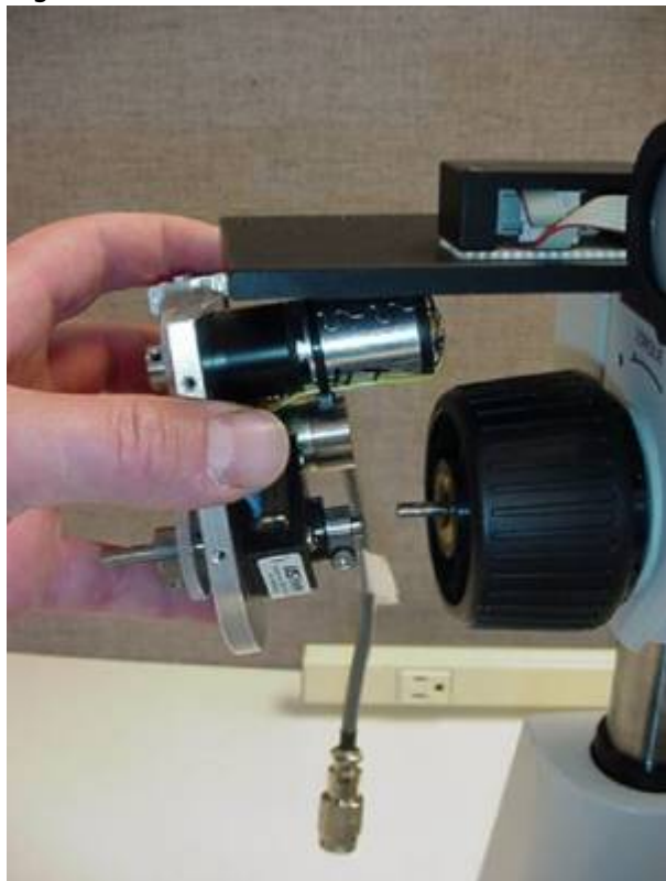
Figure 6: Install Z-drive over fine focus shaft.
