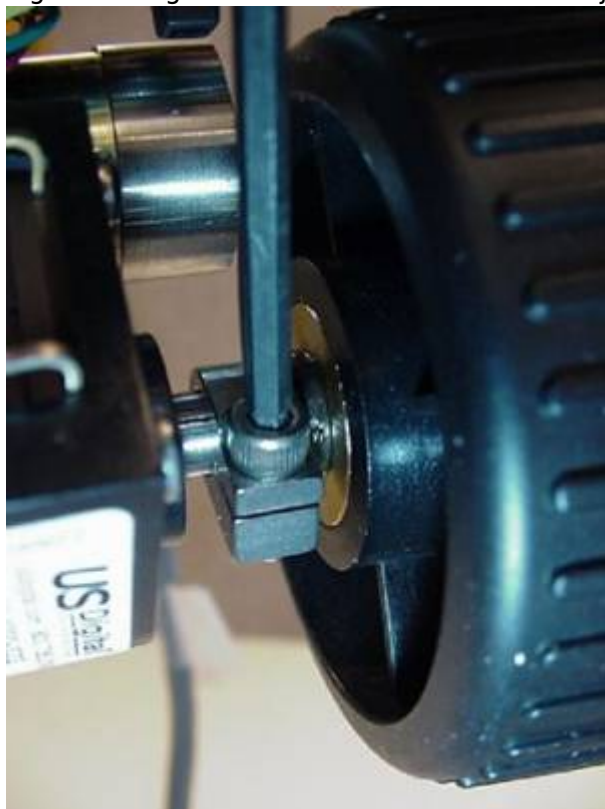
Figure 8: Push drive clamp up against focus knob & tighten
