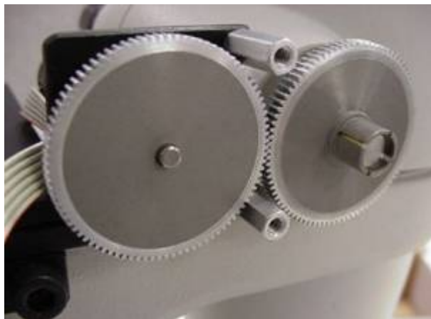
Figure 14. Gears properly aligned. . If the gears do not mate as shown loosen the thumbscrew that secures the zoom assembly to the stand, and turn the zoom assembly until the gears mate as shown. Retighten the thumbscrew when complete.
