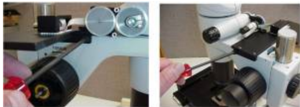
Figure 5a: Use the two 5X16mm socket head cap screws to secure the baseplate to the microscope
