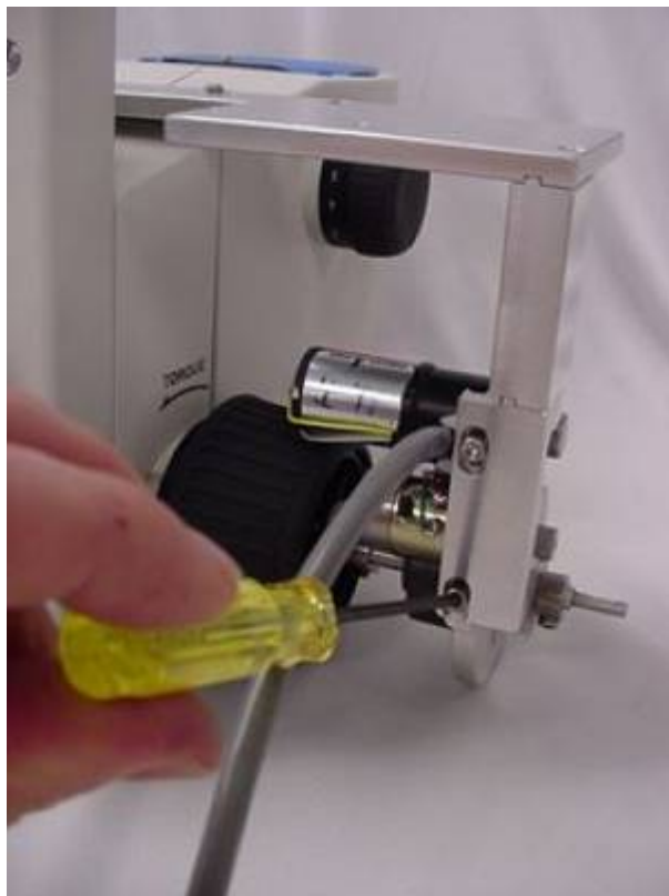
Figure 13. Tighten the vertical adjustment screws
