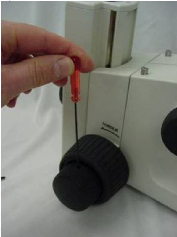
Figure 1b remove left fine focus & zoom knobs
