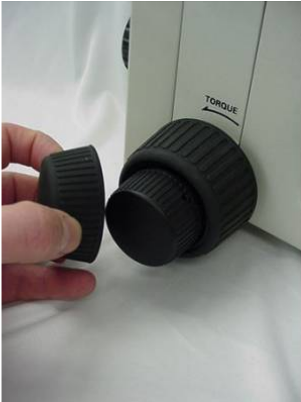
Figure 1a remove left fine focus & zoom knobs
