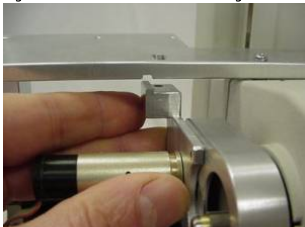
Figure 19. When gears are properly aligned use the 7/64" Allen wrench to tighten the screw that secures the zoom motor.
