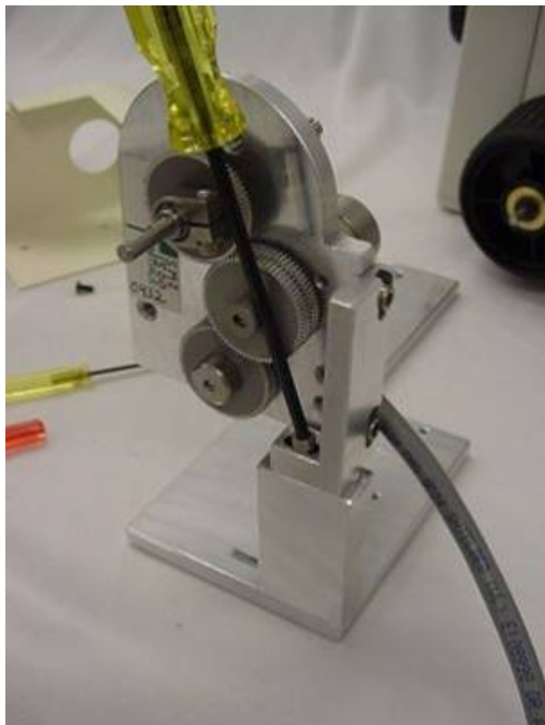
Figure 2. Removing Horizontal adjustment screw to remove Z-drive from base plate
