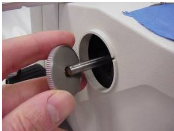
Figure 15. Installing zoom gear & spacer onto zoom shaft
