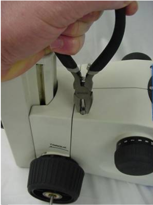
Figure 6. Use the pliers to lightly tighten the two standoffs .
