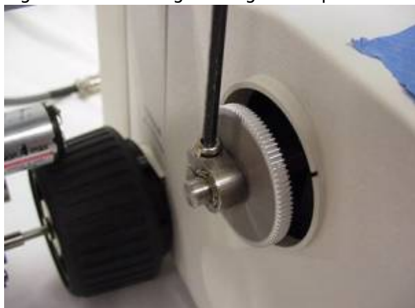
Figure 16. From the end of the zoom gear there should be a distance of \frac{3}{16} " ( \sim 4.5 mm) to the end of the shaft. Install & tighten the clamp as shown to secure the gear in place
