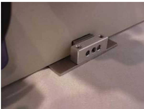
Figure 10: Tightening the base plate clamp
