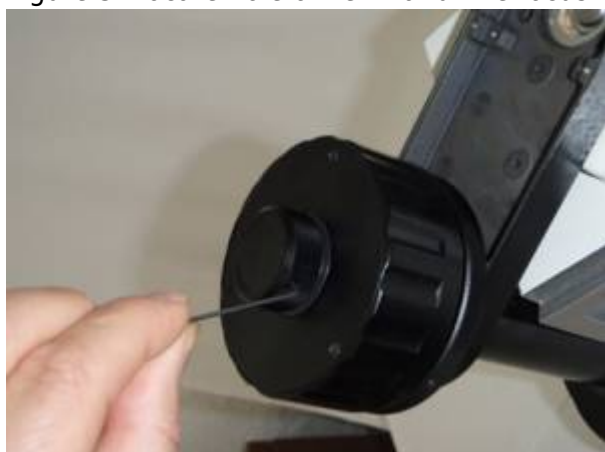
Figure 3. Locate hole on left hand fine focus knob to access setscrew
