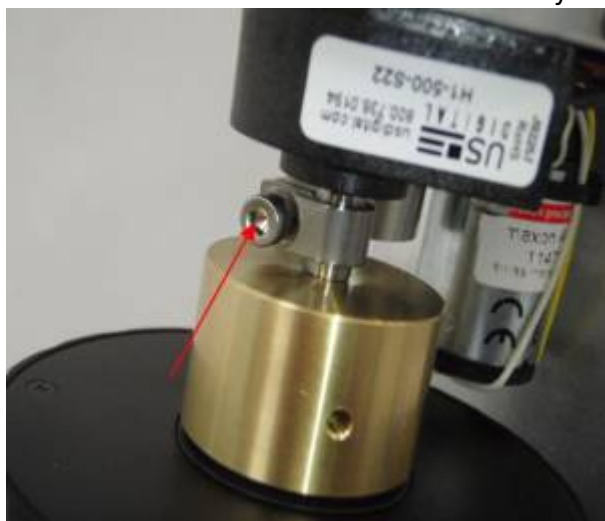
Figure 16. Use the 7/64 inch Allen wrench to securely tighten the screw on the drive shaft clamp. This is the same screw that was loosened in figure 11.
