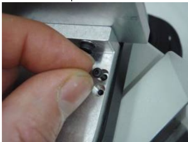
Figure 15a. Use the two 2 x 8 mm socket head cap screws sent with the drive assembly & the 1.5 mm Allen wrench to secure the drive assembly to the focus assembly as shown.
