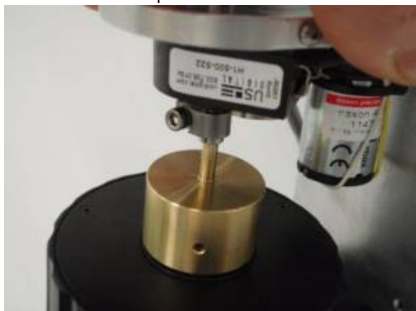
Figure 14b. Install the Z drive as shown note that the drive shaft on the drive slides over the shaft on the brass clutch plate as shown.
