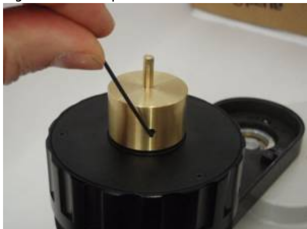
Figure 9. Use the 1.3 mm Allen wrench to tighten the setscrew securely.
