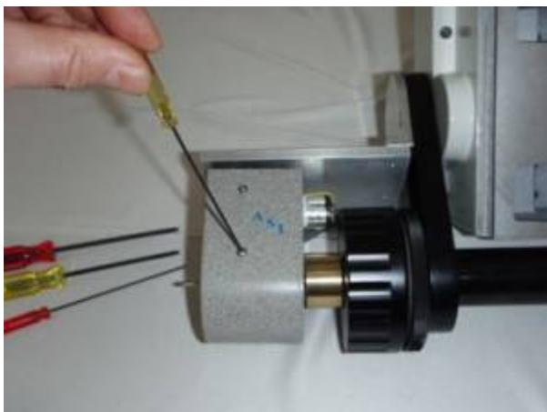
Figure 17c. Use the 1/16-inch Allen wrench to remove the two cover screws & slide the cover on as shown. Use these screws to secure the cover in place
