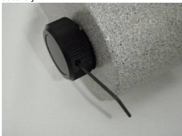
Figure 18b. Install the original knob that was removed in figure 5. Note that the setscrew must be lined up with flat on fine focus shaft as shown. Use the 1.3 mm Allen wrench to tighten the setscrew securely.
