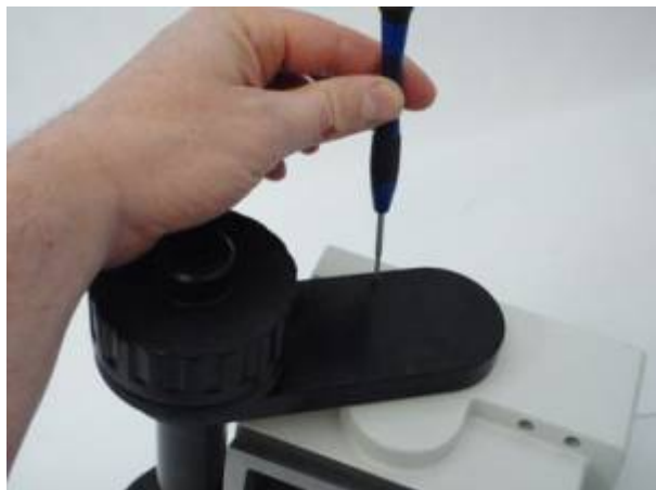
Figure 1. Locate two cross head screws that secure left hand cover & remove them .
