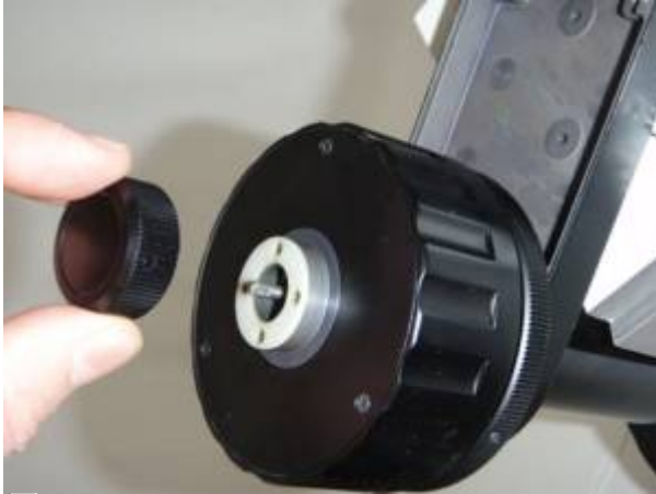
Figure 5. Pull knob off to remove it.
