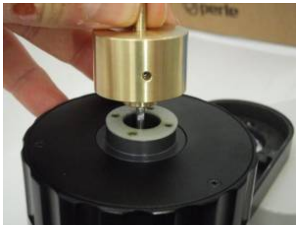
Figure 8. Install plate as shown with setscrew lined up with flat on fine focus shaft.
