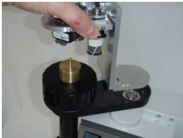
Figure 14a. Install the Z drive as shown note that the drive shaft on the drive slides over the shaft on the brass clutch plate as shown.
