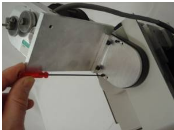
Figure 15b. Use the two 2 x 8 mm socket head cap screws sent with the drive assembly & the 1.5 mm Allen wrench to secure the drive assembly to the focus assembly as shown.
