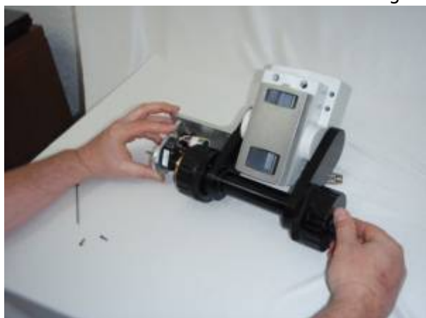
Figure 17. Slide the motor drive up and down, forward and backward slightly while turning the right fine focus knob until it is in the position where minimum drag is felt on the right focus knob. Secure the motor drive into position by tightening the horizontal and vertical adjustment screws that were loosened in figures 12 & 13. Please note that these screws should not be over tightened. In fact, the horizontal and vertical adjustment screws can be a bit loose. Recheck the z drive for drag by turning the right fine focus knob; no noticeable drag should be felt. Repeat the above steps, if necessary.
