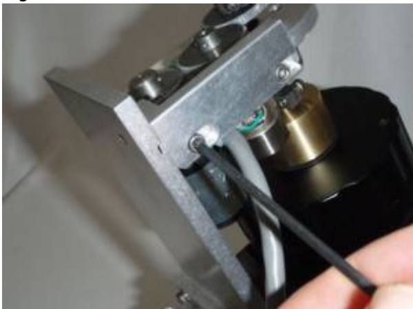
Figure 12. Use the 7/64 inch Allen wrench to loosen the vertical adjustment screws.
