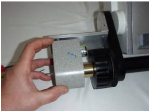
Figure 17b. Use the 1/16-inch Allen wrench to remove the two cover screws & slide the cover on as shown. Use these screws to secure the cover in place
