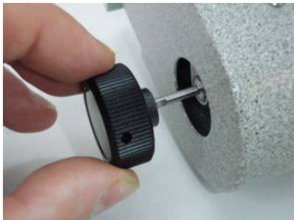
Figure 18a. Install the original knob that was removed in figure 5. Note that the setscrew must be lined up with flat on fine focus shaft as shown. Use the 1.3 mm Allen wrench to tighten the setscrew securely.
