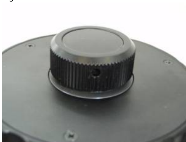
Figure 3. Locate hole on left hand fine focus knob to access setscrew
