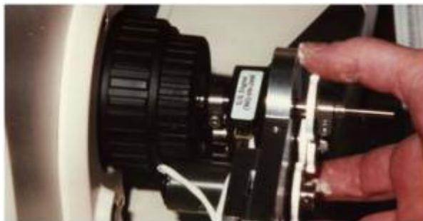
Orient the motor assembly so that the two shafts are aligned, then push the motor assembly onto the
