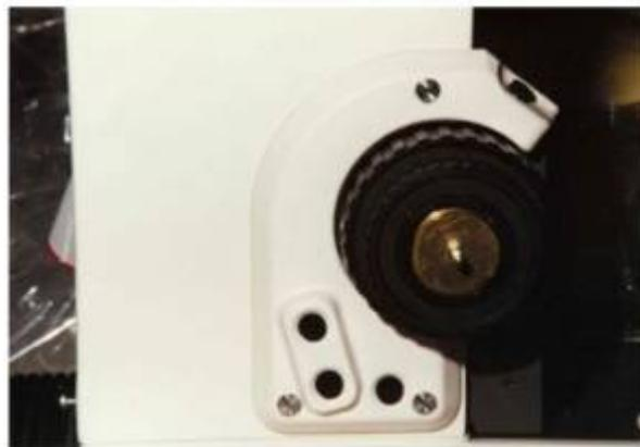
On the Microphot FXA remove the left fine focus knob by loosening the 1.5 hex head set screw that secures it to the fine focus shaft and pull the knob straight off of the shaft.
