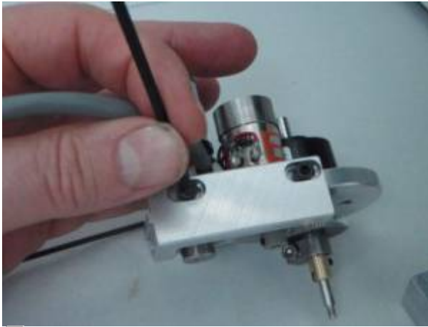
Figure 6: Location of vertical adjustment screws
