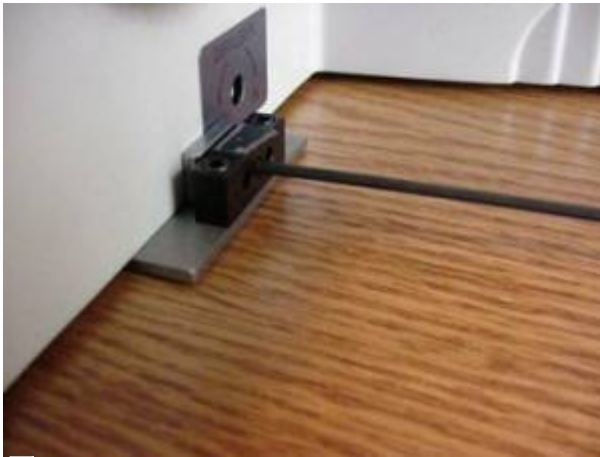
Figure 9: Tighten Baseplate set screw
