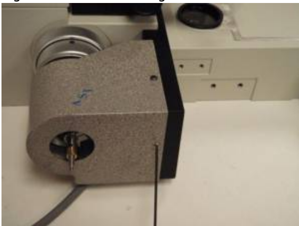
Figure 10c: Secure using 2mm Allen wrench
