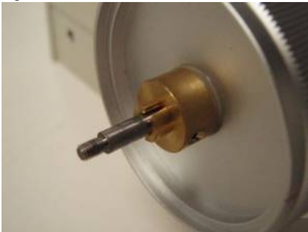
Figure 2: Pull knob straight off to expose shaft
