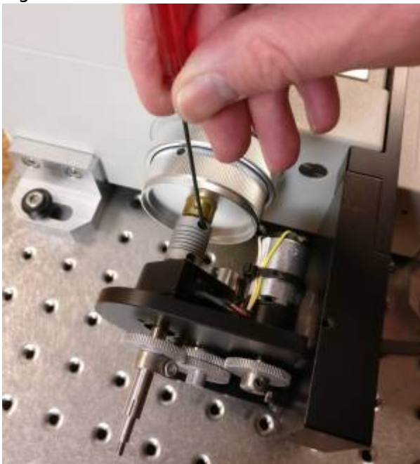
Figure 9b: Securely tighten the Flex coupler using 1.5mm Allen wrench
