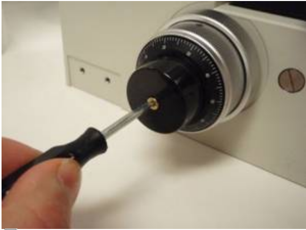
Figure 1: Pull off the Rubber Boot to expose the nut. Use screwdriver to remove the nut
