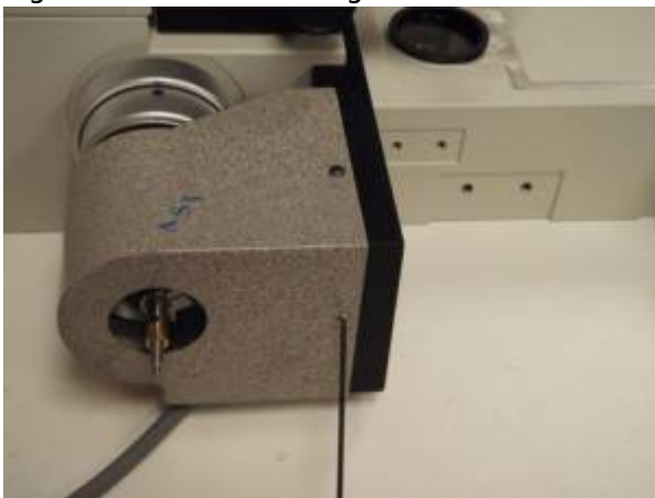
Figure 10c: Secure using 2mm Allen wrench
