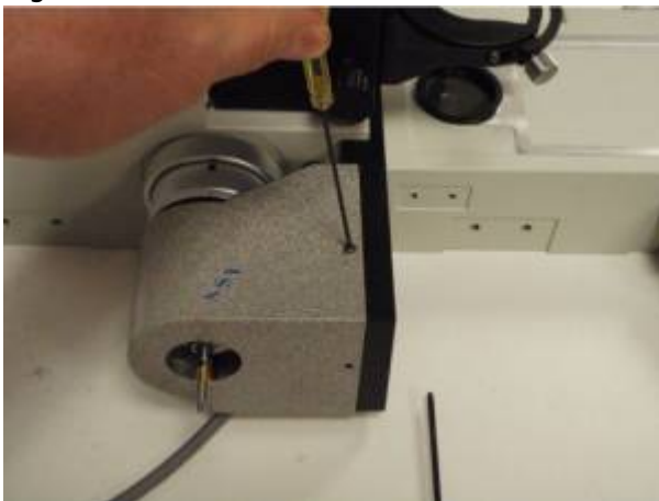
Figure 10b: Secure using 2mm Allen wrench
