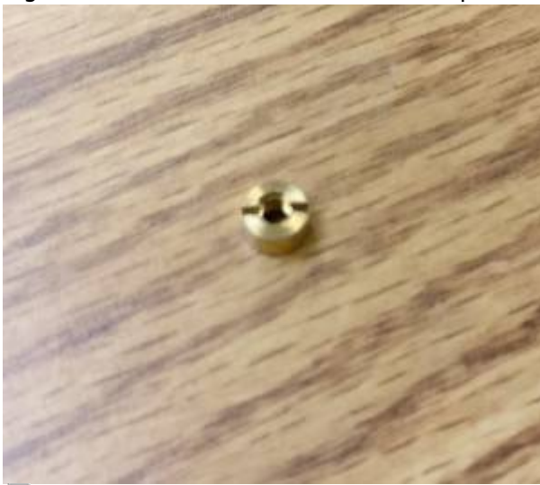
Figure 1b: Slotted Nut
