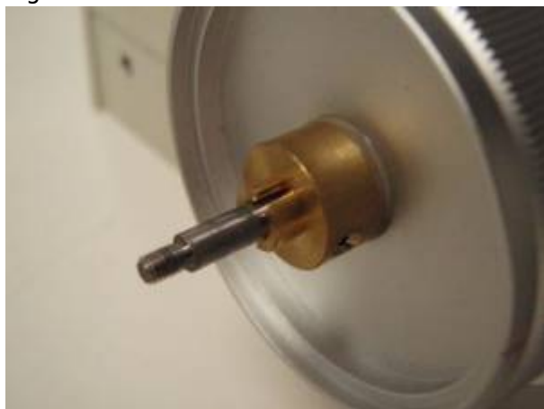
Figure 2: Pull knob straight off to expose shaft
