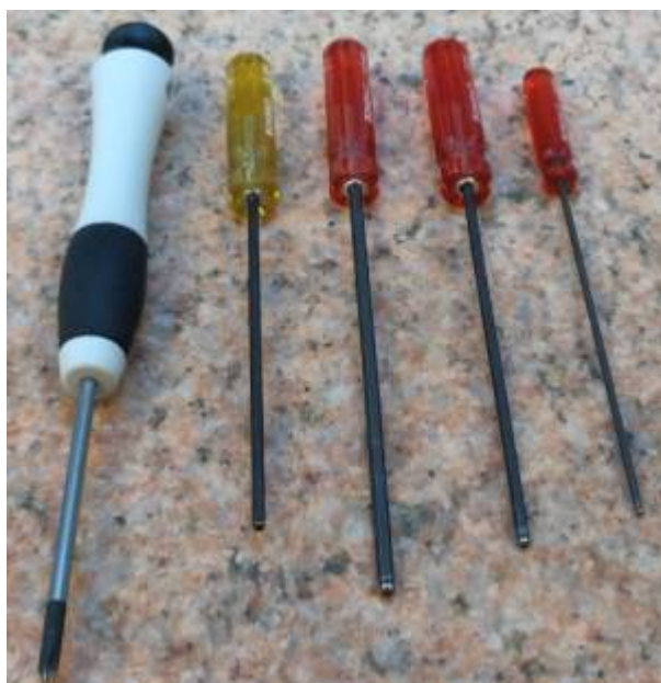
Phillips head screwdriver and 2.5 mm, 2 mm, 1.5 mm, 5/64" hex drivers
